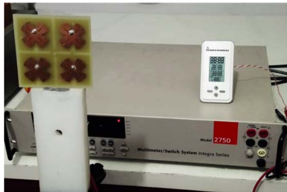
Figure 18. Rectenna used as a power supply to an LCD clock.
