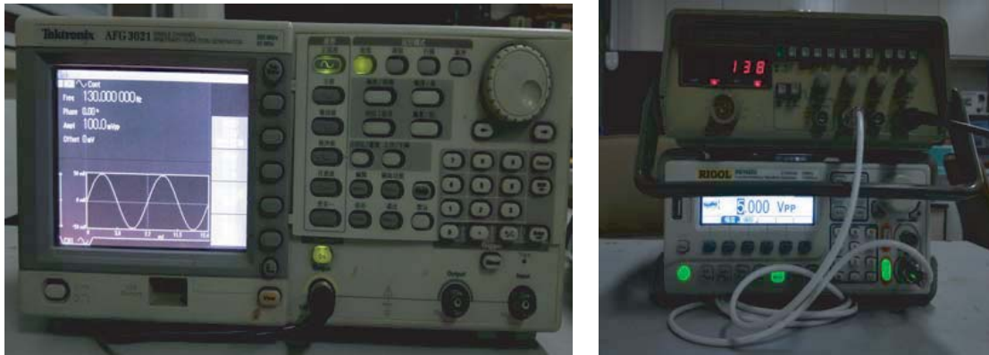
Figure 5. The physical structure of signal generators (The signal generator in left side generates the desired signal, and the others in right side generate the random phase modulation interference).
