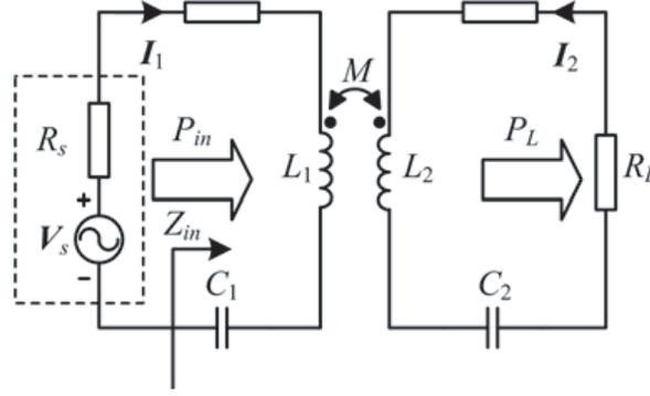
**Figure 1.** Equivalent circuit of the MCR-WPT system.
