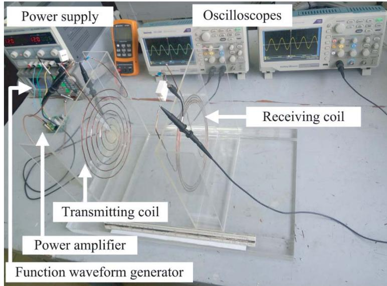
Figure 5. Prototype of the MCR-WPT system.
