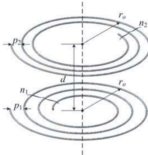
**Figure 2.** Configuration of coils in the conventional system.
