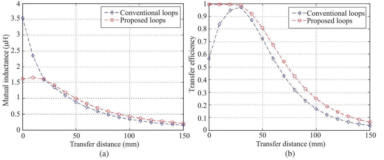
**Figure 3.** Comparisons of (a) mutual inductance, (b) transfer efficiency.
