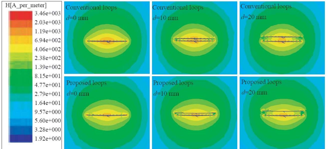
**Figure 4.** Comparisons of magnetic field distribution.
