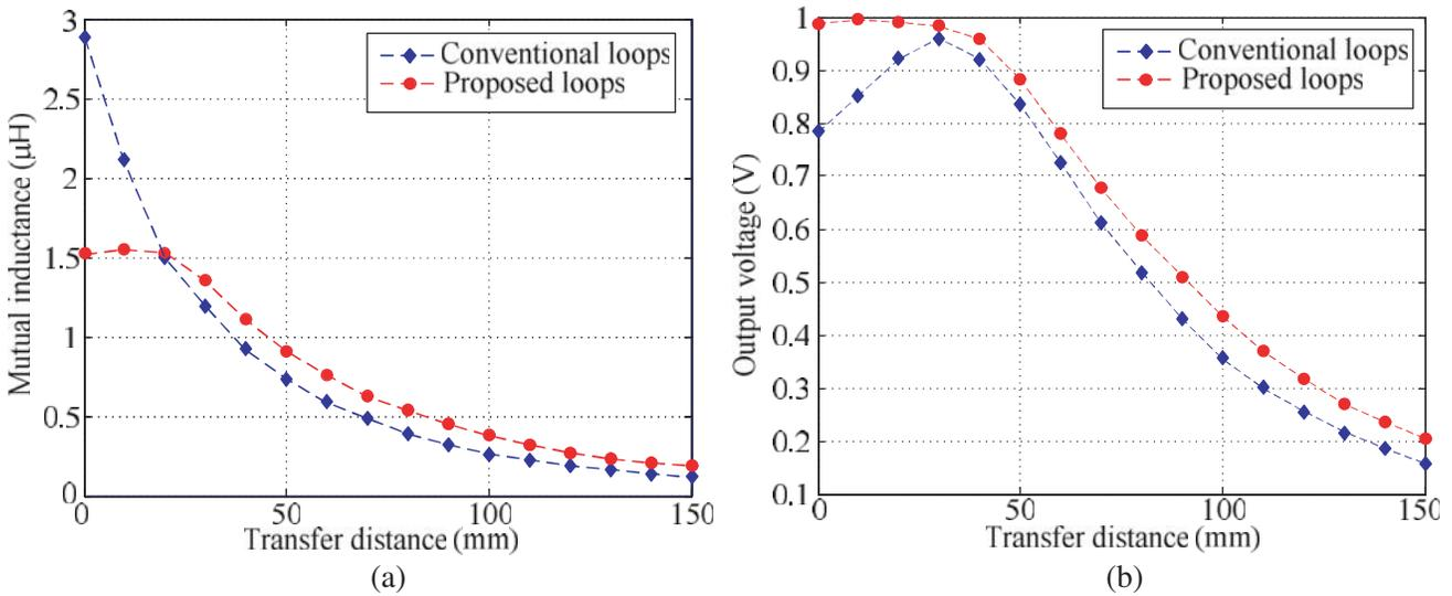
Figure 6. Comparisons of measured (a) mutual inductance, (b) output voltage.
