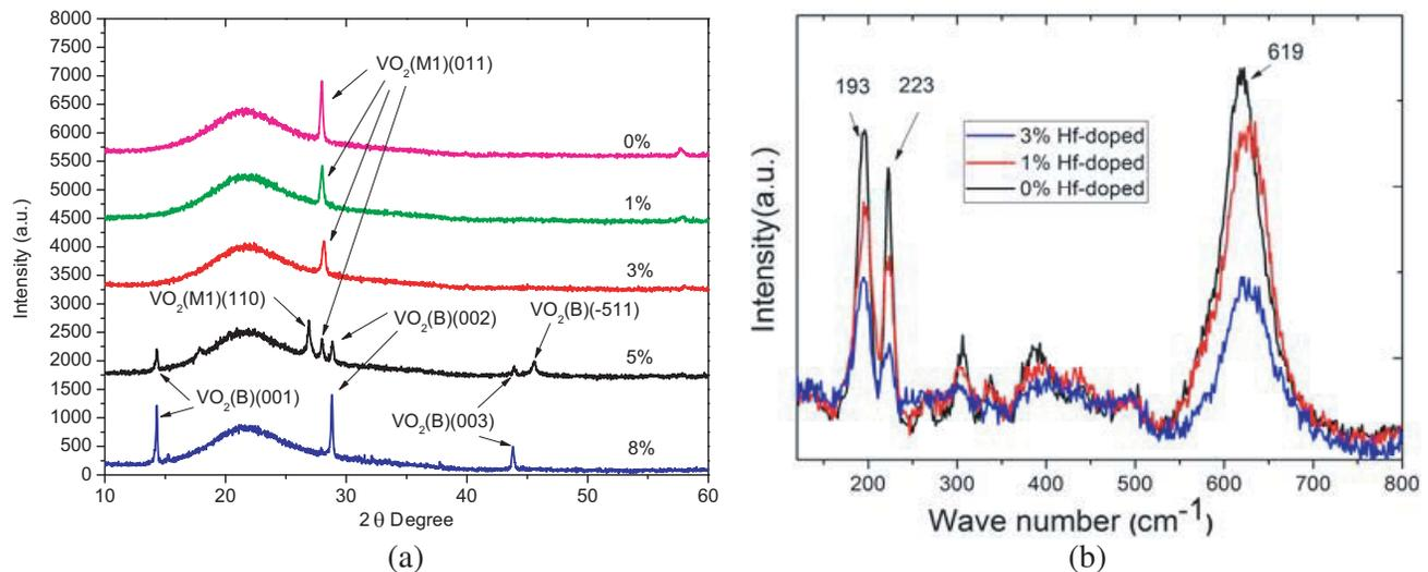
**Figure 2.** (a) XRD spectra of different concentrations of Hf-doped Vanadium dioxide films. (b) Raman spectra of different concentrations of Hf-doped Vanadium oxide films.
