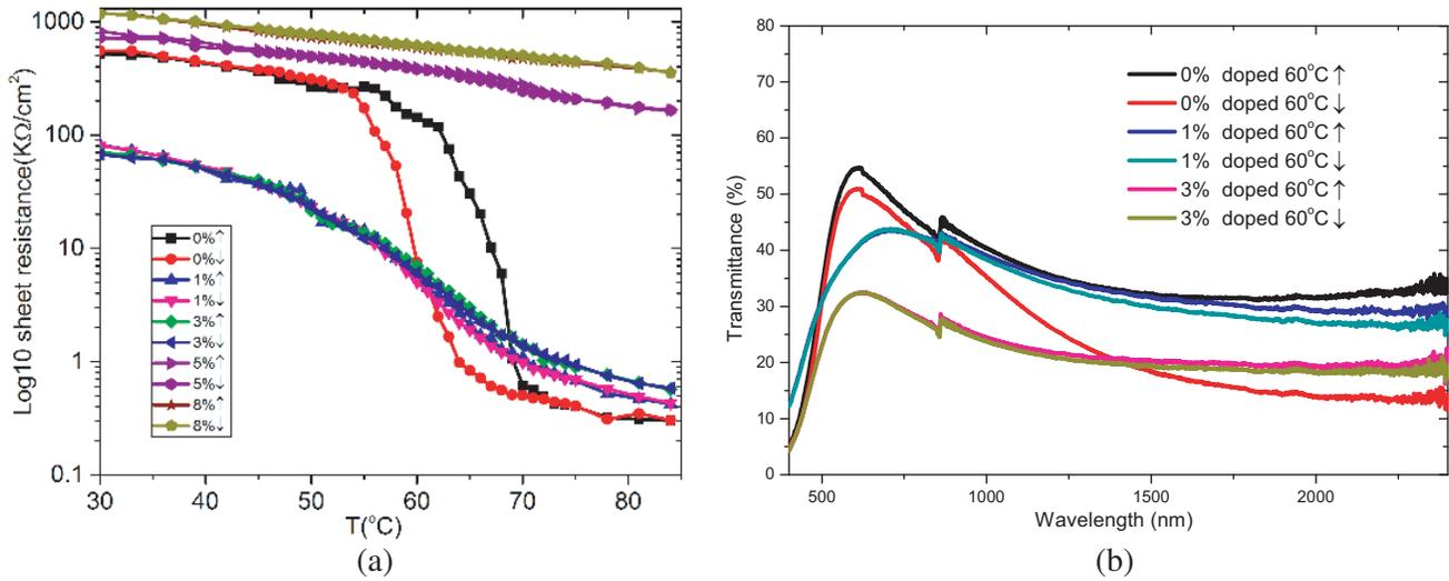
**Figure 3.** (a) Temperature dependent sheet resistance of the Hf:VO<sub>2</sub> thin films during heating and cooling processes; (b) Comparison of the transmittance spectrum of pure VO<sub>2</sub> and Hf-doped VO<sub>2</sub> thin films at 60°C during heating and cooling processes respectively.
