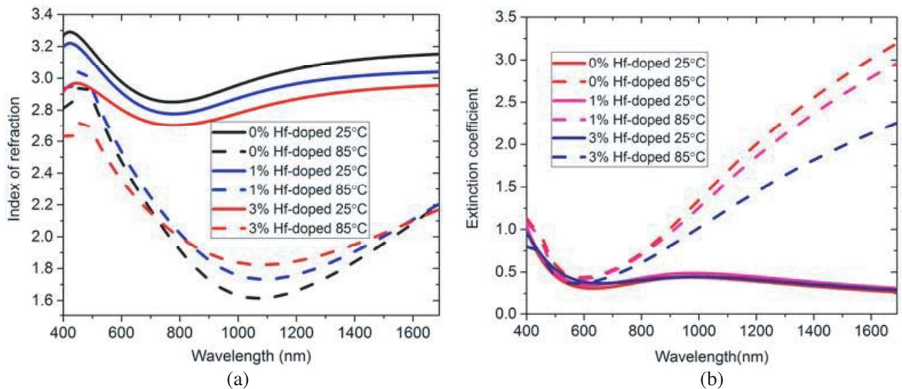
**Figure 4.** (a) Refractive index and (b) extinction ratio of different concentrations of Hf doped VO<sub>2</sub> thin films at 25°C and 85°C.
