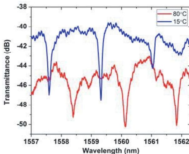
**Figure 6.** Resonance peaks at device temperatures of 15°C and 80°C.
