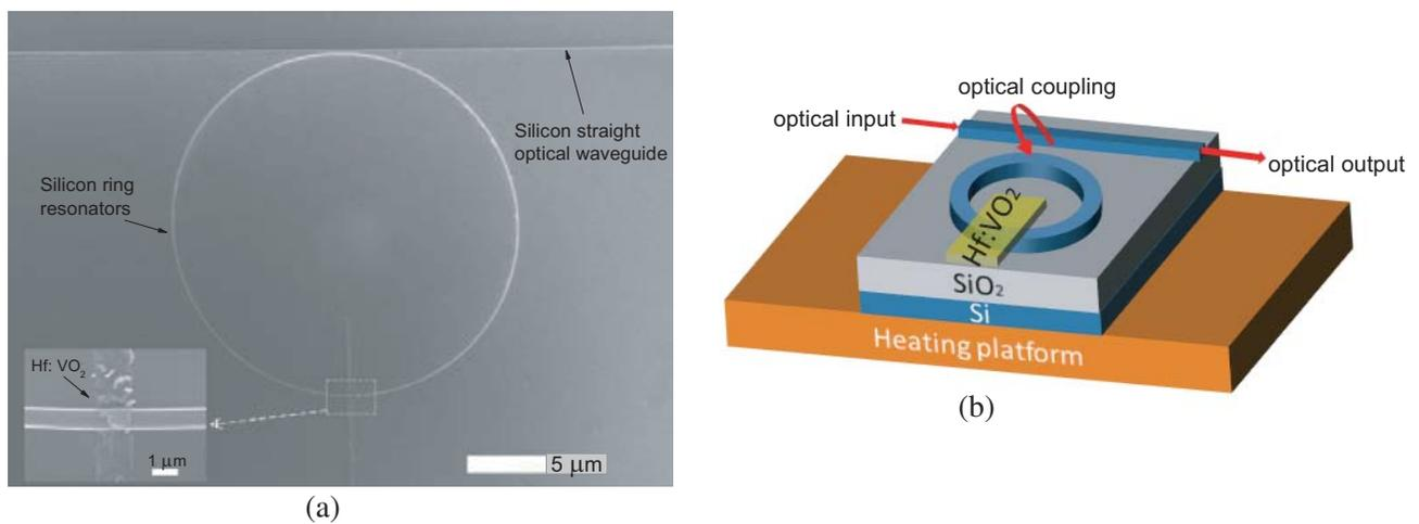
**Figure 5.** (a) SEM image of silicon ring resonator device partially covered by 3% Hf-doped vanadium oxide thin films. (b) The schematic characterization approach of the transmittance spectrum of the device. The heating of device was executed via a heating platform. After light inputting the silicon straight optical waveguide, the light of particular wavelength will be coupled into Silicon ring resonator device, causing no optical output of counterparts.
