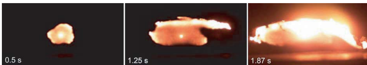
Figure 2. Frames of high-speed imaging of Al nanopowder combustion in its own light at different moments of time, relative to the ignition moment.
