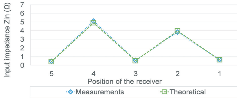
Figure 7. \hat{Z}_{in}(\Omega) at the resonant frequency f_0 = 147 kHz obtained with measurement using the VNA and with Eq. (6) using Eq. (3) versus different positions of the receiver.
