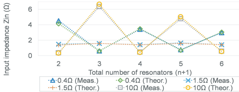
Figure 6. \hat{Z}_{in} ( \Omega ) at the resonant frequency f_0 = 147 kHz obtained with measurements with VNA and with Eq. (6) using Eq. (2) for different values of R'_T ( 0.4 \Omega , 1.5 \Omega and 10 \Omega ) and different number of resonators.
