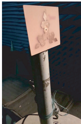
Figure 11. Radiation pattern measurement of proposed ASFM-Antenna using anechoic chamber.
