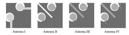
Figure 2. Design process of the proposed UWB MIMO antenna.
