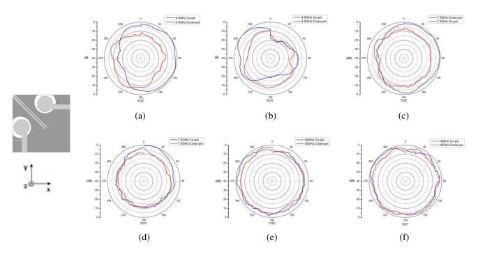
**Figure 7.** Measured radiation patterns of the proposed antenna: (a) 4.5 GHz YZ-plane, (b) 4.5 GHz XZ-plane, (c) 7.5 GHz YZ-plane, (d) 7.5 GHz XZ-plane, (e) 10 GHz YZ-plane, (f) 10 GHz XZ-plane.
