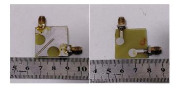
Figure 5. Fabricated prototype of proposed antennas.
