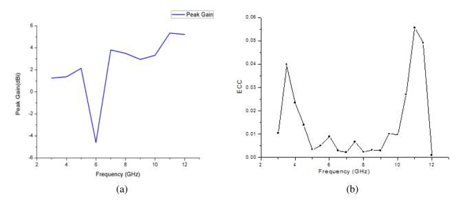
Figure 8. (a) Measured peak gains of proposed antenna and (b) ECC of the proposed antenna.
