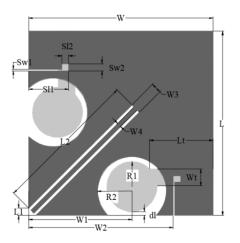
Figure 1. Geometry of the proposed UWB MIMO antenna.
