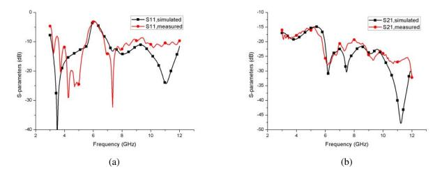
**Figure 6.** Measured and simulated S-parameters of proposed antenna: (a)  $S_{11}$  and (b)  $S_{21}$ .
