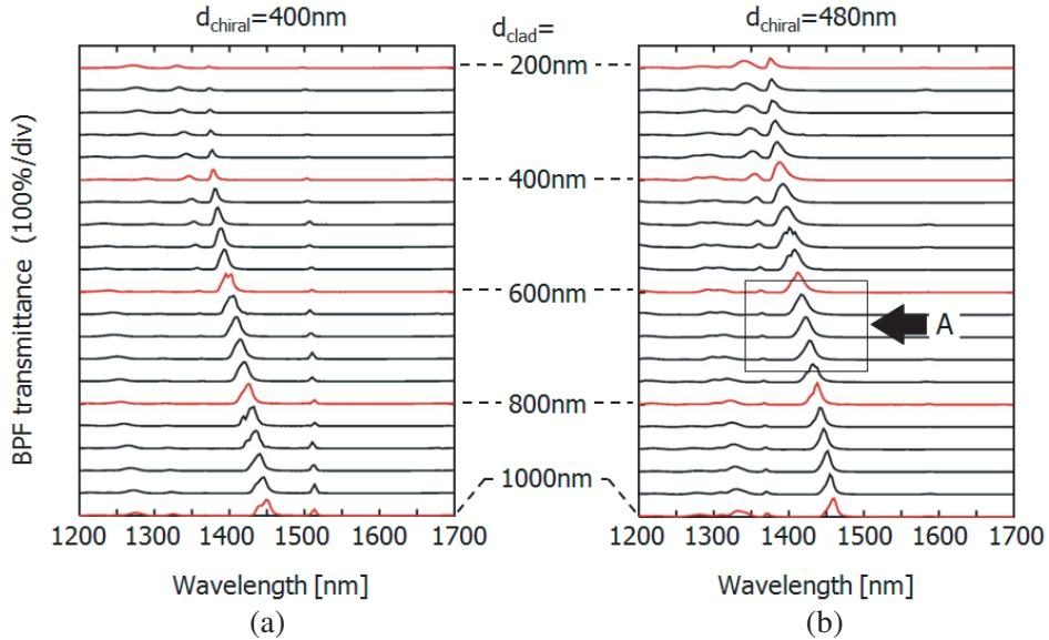
**Figure 6.** Calculated transmission spectra of BPFs using Si/Al<sub>2</sub>O<sub>3</sub> PCM. (a) Thin Si chiral layer ( $d_{\text{chiral}} = 400 \text{ nm}$ ) case. Each plot correspond to different underclad thickness. (b) Thick ( $d_{\text{chiral}} = 480 \text{ nm}$ ) Si chiral layers. Region A indicates the unimodal construction. Grating period was fixed as  $\Lambda = 960 \text{ nm}$ .
