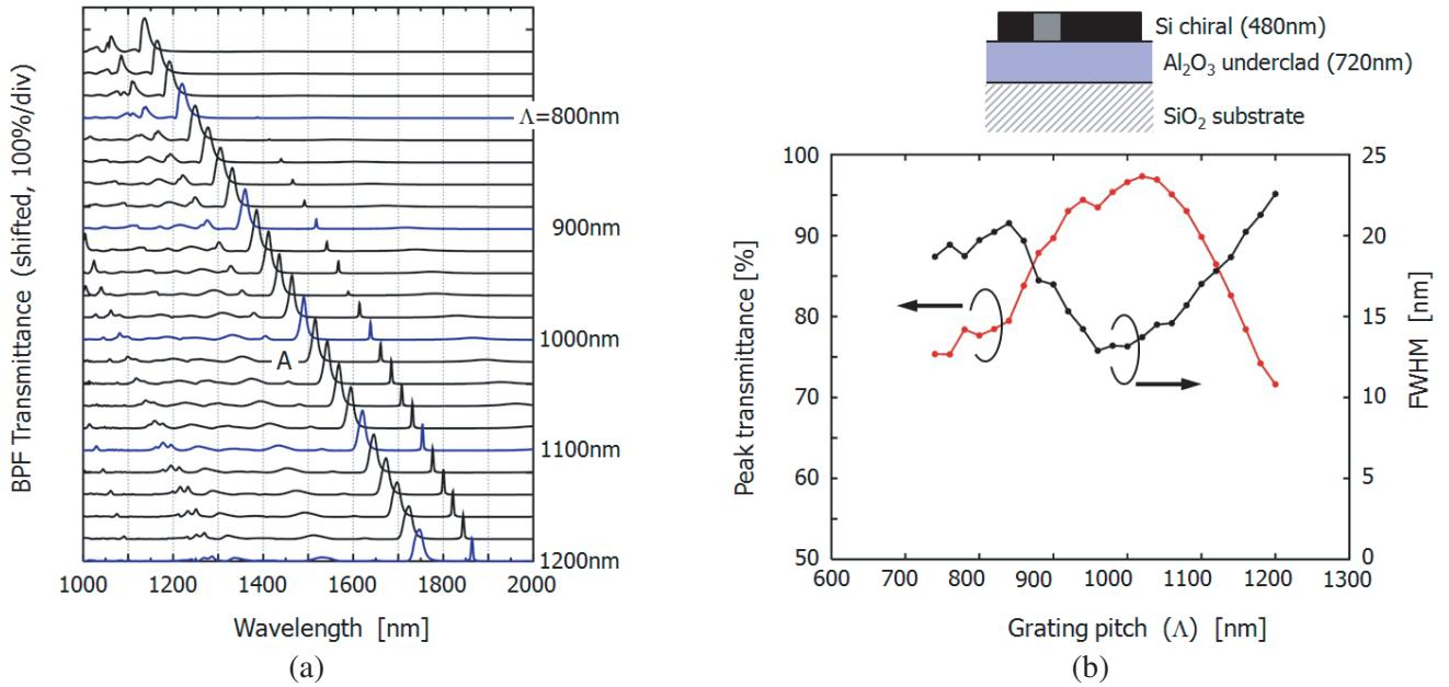
**Figure 7.** Designed single-peak filtering characteristics of Si/ $\text{Al}_2\text{O}_3$  PCM. (a) Spectra for various grating period ( $\Lambda$ ). Thickness of Si chiral and  $\text{Al}_2\text{O}_3$  underclad layers are  $600 \text{ nm}$  and  $540 \text{ nm}$ , respectively. (b) Transmittance and bandwidth of the transmission peak ‘A’ in the left figure.
