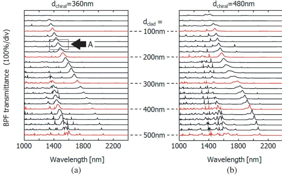
**Figure 8.** Calculated transmission spectra of BPFs using partially-etched type Si PCM. (a) Thin Si chiral layer ( $d_{\text{chiral}} = 360 \text{ nm}$ ) case. Each plot correspond to different “unetched” Si thickness. Region A indicates high transmittance and almost unimodal construction. (b) Thick ( $d_{\text{chiral}} = 480 \text{ nm}$ ) chiral layer. Grating period was fixed as  $\Lambda = 960 \text{ nm}$ .
