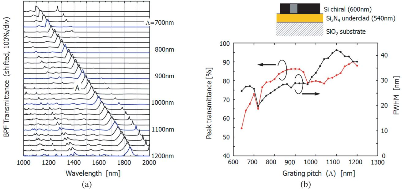
**Figure 5.** Designed single-peak filtering characteristics of Si/Si<sub>3</sub>N<sub>4</sub> PCM. (a) Spectra for various grating period ( $\Lambda$ ). Thickness of Si chiral and Si<sub>3</sub>N<sub>4</sub> underclad layers were 600 nm and 540 nm, respectively. (b) Maximum transmittance and bandwidth of the main peak (indicated as ‘A’ in the left figure).
