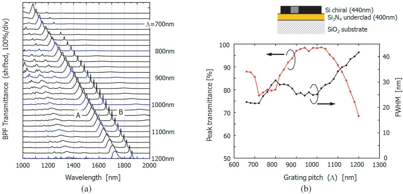
**Figure 4.** Designed double-peak filtering characteristics of  $\text{Si}/\text{Si}_3\text{N}_4$  PCM. (a) Spectra for various grating period ( $\Lambda$ ). Thickness of Si chiral and  $\text{Si}_3\text{N}_4$  underclad layers were 440 nm and 400 nm, respectively. (b) Transmittance and bandwidth of the main peak (indicated as 'A' in the left figure).
