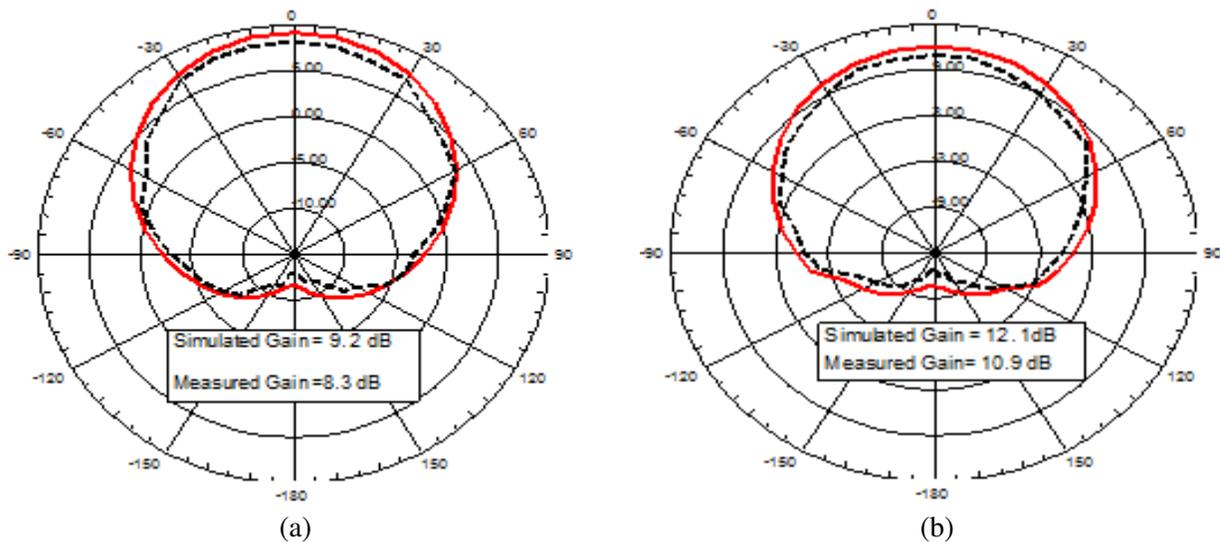
**Figure 7.** Gain comparison plot between simulated and measured values of hybrid antenna mounted on the cylindrical surface at 1000 mm diameter. (a) Single antenna. (b) Dual antenna.
