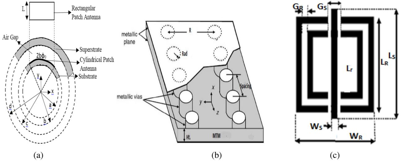
**Figure 2.** (a) Cylindrical-rectangular microstrip antenna with superstrate gap. (b) SIW with cylindrical metallize vias. (c) MTM using split rectangular ring resonator with metallic wire strip.
