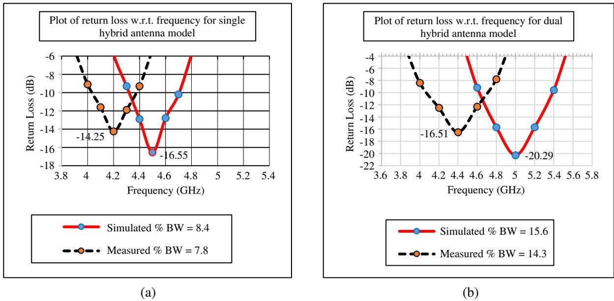
**Figure 6.** Bandwidth comparison plot between simulated and measured values of hybrid antenna mounted on the cylindrical diameter at 1000 mm surface. (a) Single antenna. (b) Dual antenna.
