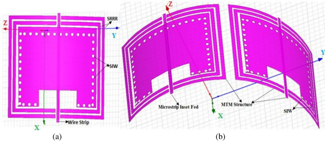
**Figure 3.** Geometry of rectangular hybrid antenna mounted on the cylindrical surface. (a) Single antenna model. (b) Dual antenna model.
