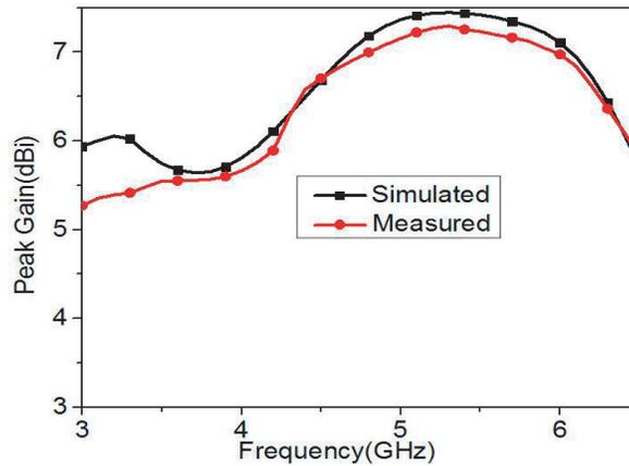
**Figure 11.** The measured and simulated antenna peak gains of the antenna.
