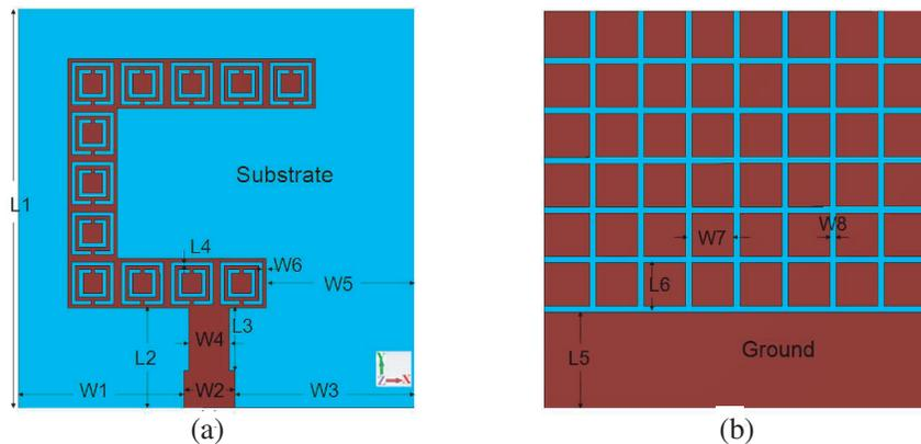
**Figure 2.** Configuration of antenna. (a) Top view. (b) Bottom view.
