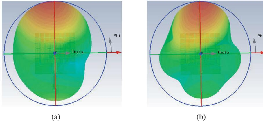
**Figure 8.** Simulated 3D radiation patterns of the proposed antenna at (a) 4.12 GHz, (b) 5.60 GHz.
