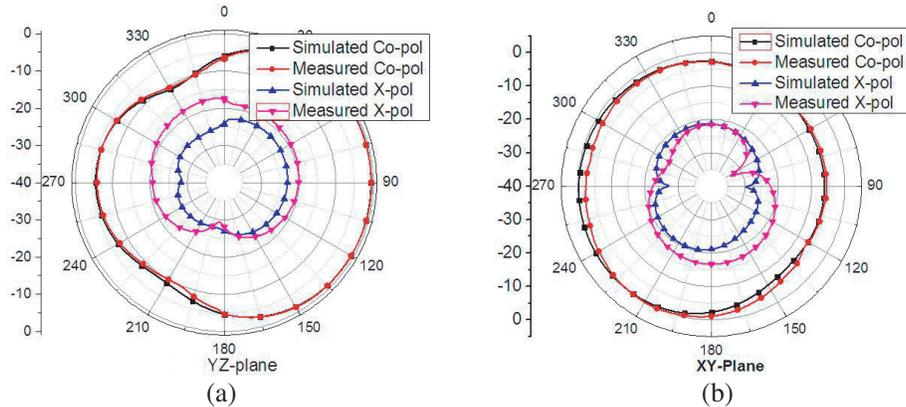
**Figure 10.** Radiation patterns of the proposed antenna at 5.60 GHz. (a)  $YZ$ -plane. (b)  $XZ$ -plane.
