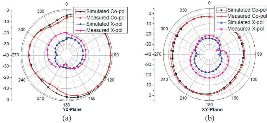
**Figure 9.** Radiation patterns of the proposed antenna at 4.12 GHz. (a)  $YZ$ -plane. (b)  $XZ$ -plane.
