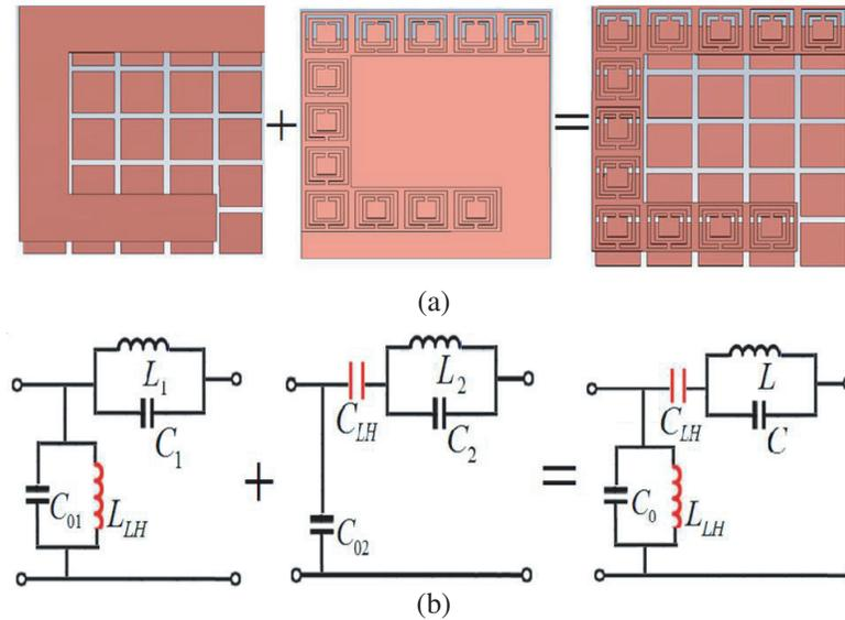
**Figure 1.** Equivalent circuit model of the MTL. (a) Configuration. (b) The relative equivalent circuit.
