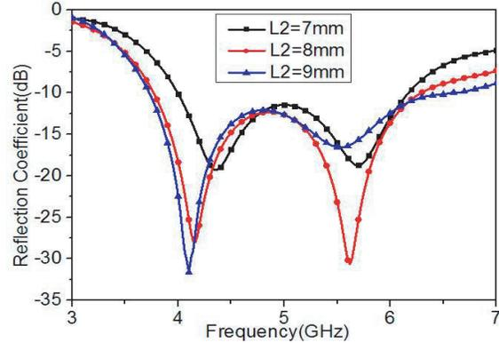
**Figure 5.** Simulated reflection coefficients curves of the proposed antenna with different  $L_2$ .
