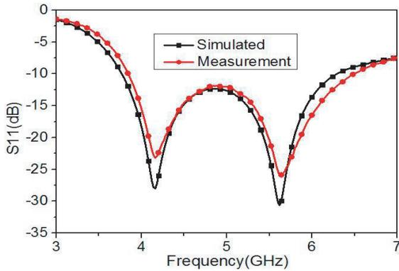
**Figure 6.** Simulated and measured reflection coefficients characteristics curves.
