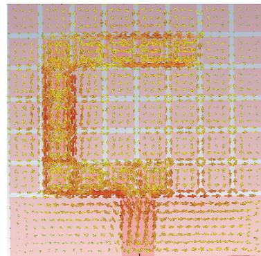
**Figure 7.** Simulated surface current distributions of the proposed antenna at 4.6 GHz.
