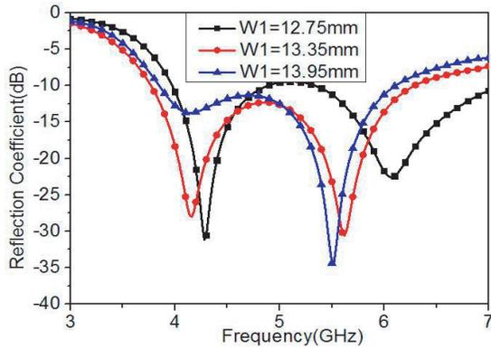
**Figure 4.** Simulated reflection coefficients curves of the proposed antenna with different  $W_1$ .
