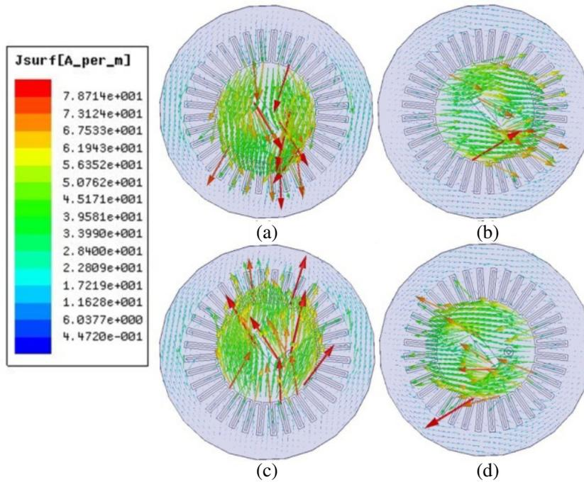
Figure 3. Current distributions of the antenna at  $TM_{11}$  mode: (a)  $t = 0$ ; (b)  $t = T/4$ ; (c)  $t = T/2$ ; (d)  $t = 3T/4$ .
