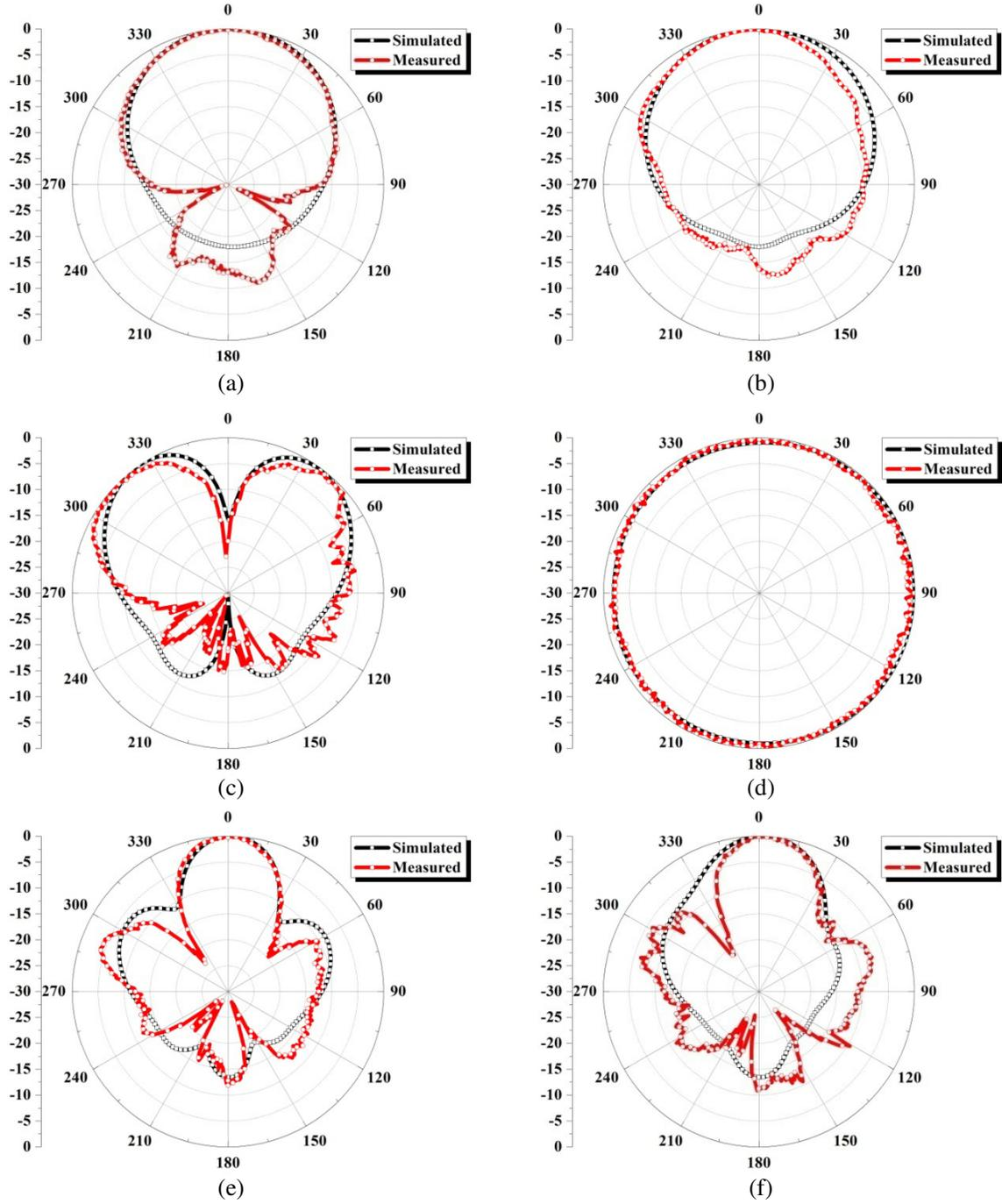
**Figure 9.** Simulated and measured radiation patterns: (a)  $E$  plane at 2.4 GHz; (b)  $H$  plane at 2.4 GHz; (c)  $E$  plane (simulated at 5 GHz, measured at 5.2 GHz); (d)  $H$  plane (simulated at 5 GHz, measured at 5.2 GHz); (e)  $E$  plane at 6.35 GHz; (f)  $H$  plane at 6.35 GHz.
