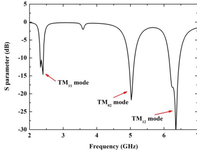
Figure 2. Simulated reflection coefficient of the antenna.
