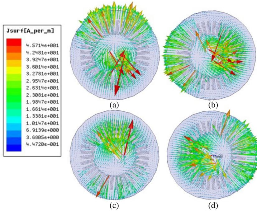
**Figure 5.** Current distributions of the antenna at  $TM_{12}$  mode: (a)  $t = 0$ ; (b)  $t = T/4$ ; (c)  $t = T/2$ ; (d)  $t = 3T/4$ .
