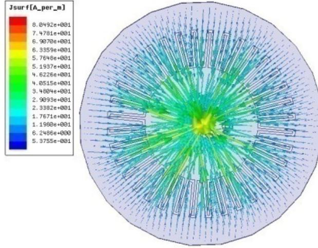
**Figure 4.** Current distribution of the antenna at  $TM_{02}$  mode.
