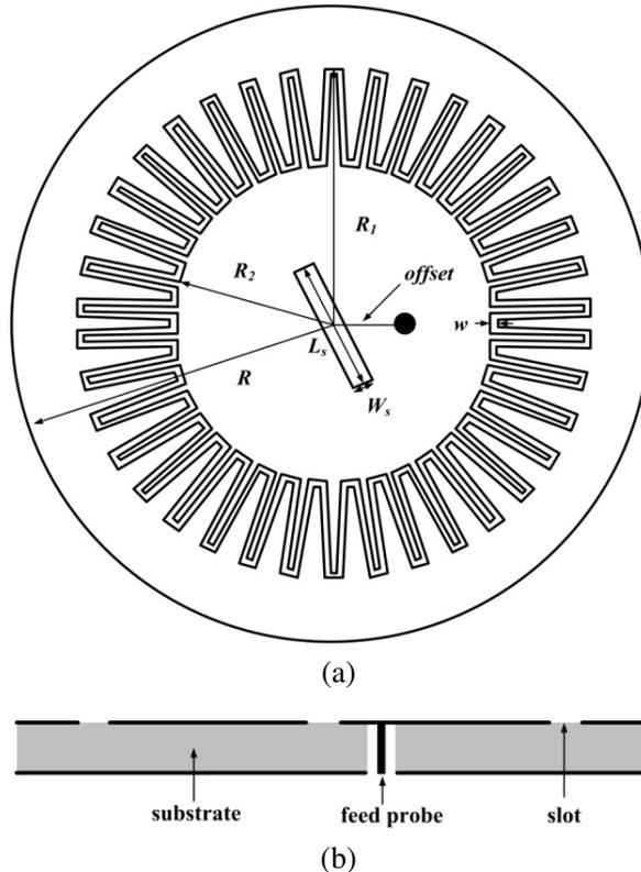
**Figure 1.** Geometry of the proposed antenna: (a) top view; (b) side view.
