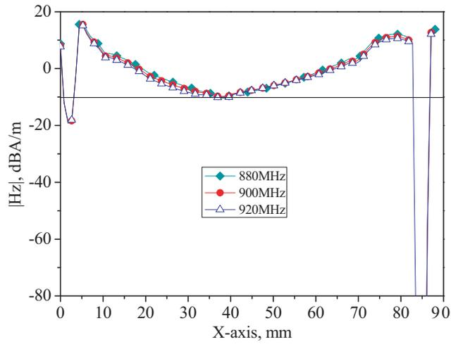
Figure 6. Simulated  $|H_z|$  along X-axis at  $Z = 5$  m.
