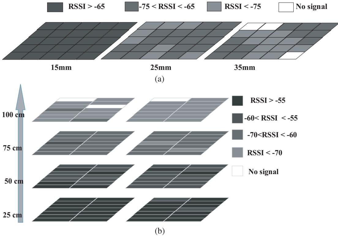
**Figure 8.** Tag detection test for NF and FF tag, by varying distance, position with respect to antenna surface. Input power has been set to 25 dBm. (a) RSSI values of near-field tags. (b) RSSI values of far-field tags along  $X$ -axis and  $Y$ -axis.
