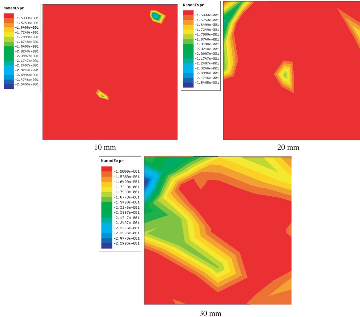
Figure 7. Simulated  $|H_z|$  distribution at  $Z = 10$  mm; 20 mm; 30 mm.
