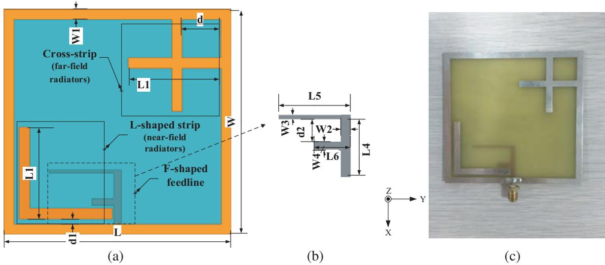
**Figure 1.** Antenna prototype. Main geometrical parameters are:  $L = W = 88$  mm,  $L1 = 36$  mm,  $W1 = 4$  mm,  $d = 15$  mm,  $d1 = 2$  mm,  $L4 = 24$  mm,  $L5 = 28$  mm,  $L6 = 11.5$  mm,  $W2 = 3$  mm,  $W3 = 1.5$  mm,  $W4 = 2.7$  mm and  $d2 = 10$  mm. (a) Top view. (b) Bottom view. (c) Physical antenna.
