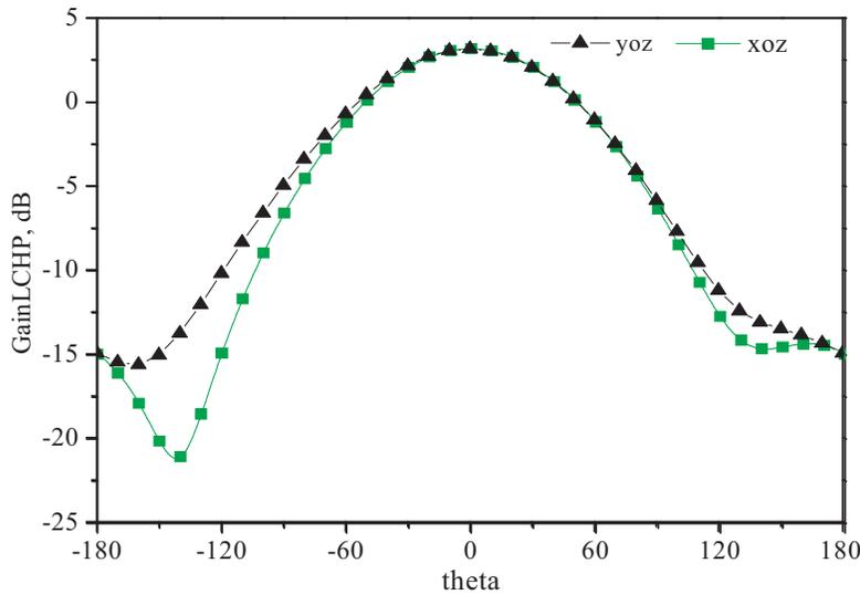
**Figure 5.** Measured Gain LCHP in  $xoz$  and  $yo z$  planes at 900 MHz.
