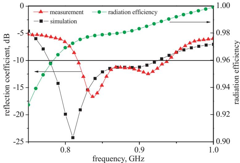
**Figure 3.** Measured reflection coefficient and radiation efficiency of proposed antenna.
