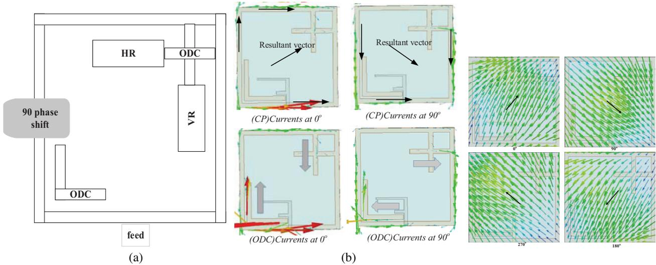
**Figure 2.** Antenna currents distribution. (a) Design thought. (b) CP and ODC currents distribution at  $0^\circ$  and  $90^\circ$  when frequency is at 900 MHz.
