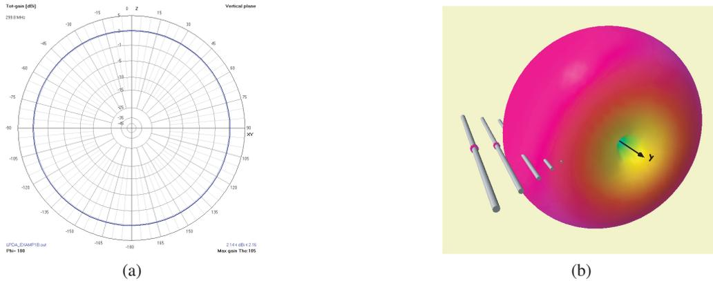
Figure 5. *H*-plane radiation pattern, 5 dipoles driven, optimized excitation.
