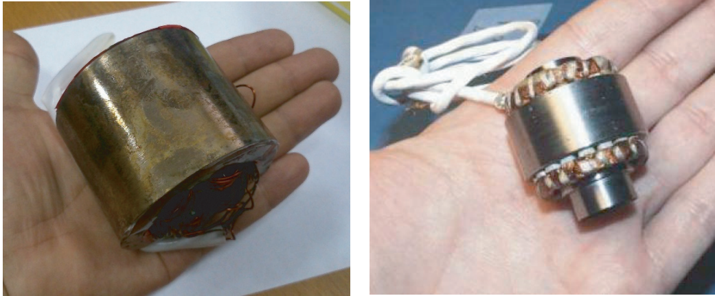
Figure 11. The designed 5 kW HSPMTC with the rotational speed of 60,000 rpm for UAV and the 1 kW HSPMTC for UAV by Hamilton Sundstrand [16].
