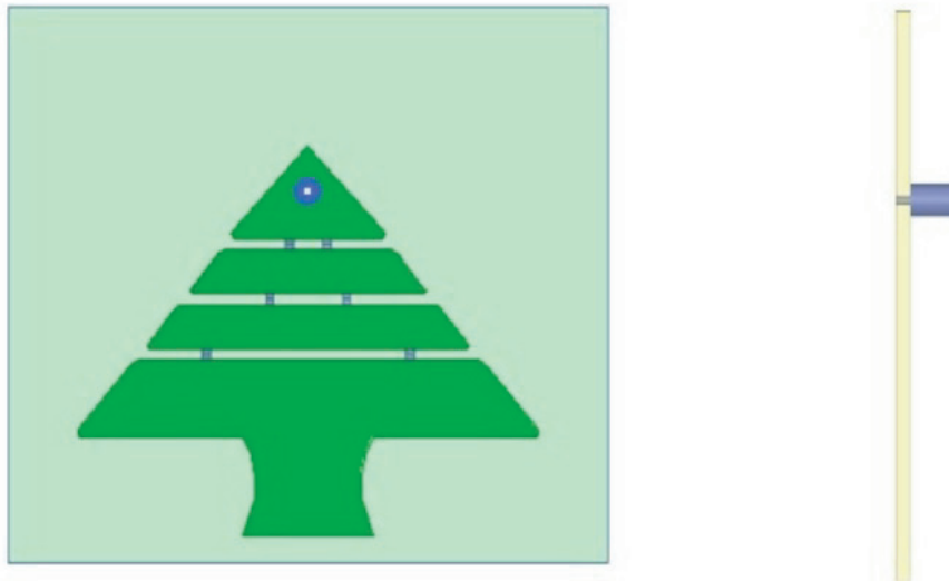
Figure 1. HFSS model of the modified cedar shape antenna showing position of the coaxial feed from a top and lateral view.
