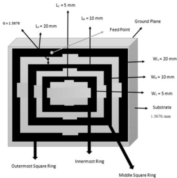
Figure 2. Square shaped fractal antenna with 2nd iteration.
