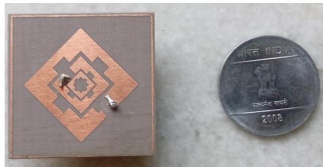
**Figure 11.** Photograph of square shaped fractal antenna with metamaterial loading.
