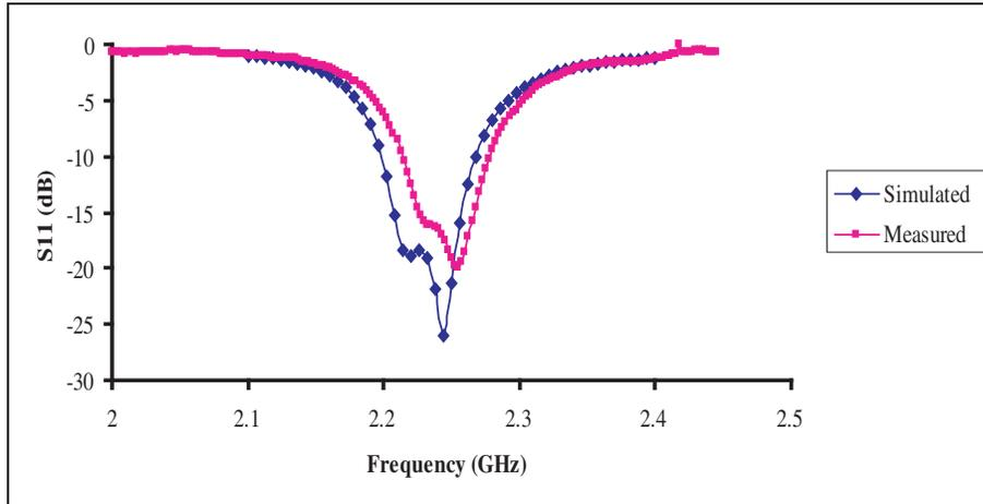
**Figure 10.**  $S_{11}$  characteristics of Koch CP antenna-3 of stage-1 simulated and measured.
