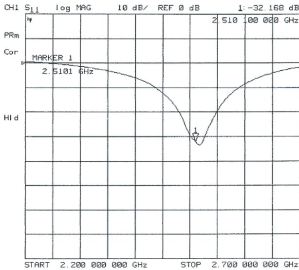
**Figure 6.** Measured  $S_{11}$  characteristics of Koch CP antenna stage-1.
