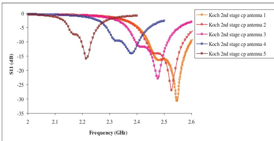
**Figure 12.**  $S_{11}$  characteristics of Koch CP 2nd stage CP antenna for different indentation angles.
