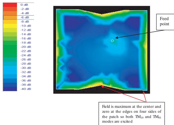
**Figure 14.** Current distribution over the patch with  $TM_{10}$  and  $TM_{01}$  modes excitation.
