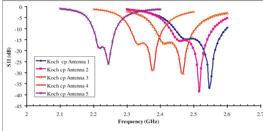
**Figure 4.**  $S_{11}$  characteristics of Koch fractal boundary CP antenna stage-1 for different indentation angles.
