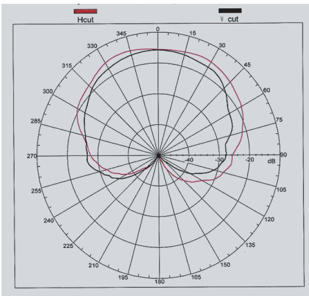
**Figure 8.** Measured radiation pattern of Koch CP antenna stage 1 in two orthogonal planes at 2510 MHz.
