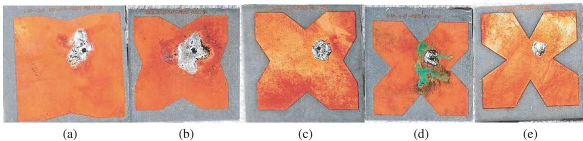
**Figure 3.** Photographs of fabricated Koch fractal boundary CP antennas stage-1. (a) Koch CP antenna 1. (b) Koch CP antenna 2. (c) Koch CP antenna 3. (d) Koch CP antenna 4. (e) Koch CP antenna 5. Koch CP antenna 1:  $13^{\circ}-0^{\circ}$ ; Koch CP antenna 2:  $30^{\circ}-20^{\circ}$ , Koch CP antenna 3:  $40^{\circ}-31^{\circ}$ , **Koch CP antenna 4:  $50^{\circ}-43^{\circ}$** , Koch CP antenna 5:  $60^{\circ}-55^{\circ}$ .
