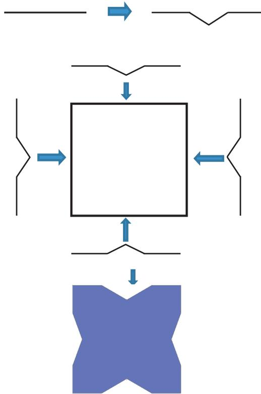
**Figure 1.** Generation of Koch fractal boundary CP antenna stage-1.
