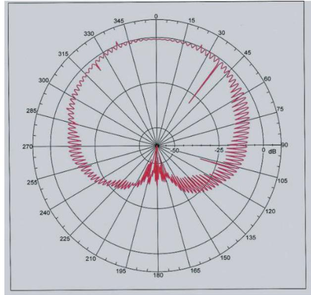
**Figure 9.** Measured Rotating linear pattern of Koch CP antenna stage 1 at 2510 MHz.
