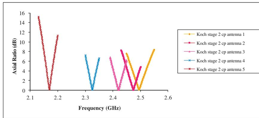
**Figure 13.** Axial ratio characteristics of Koch stage 2 CP antenna for different indention angles.
