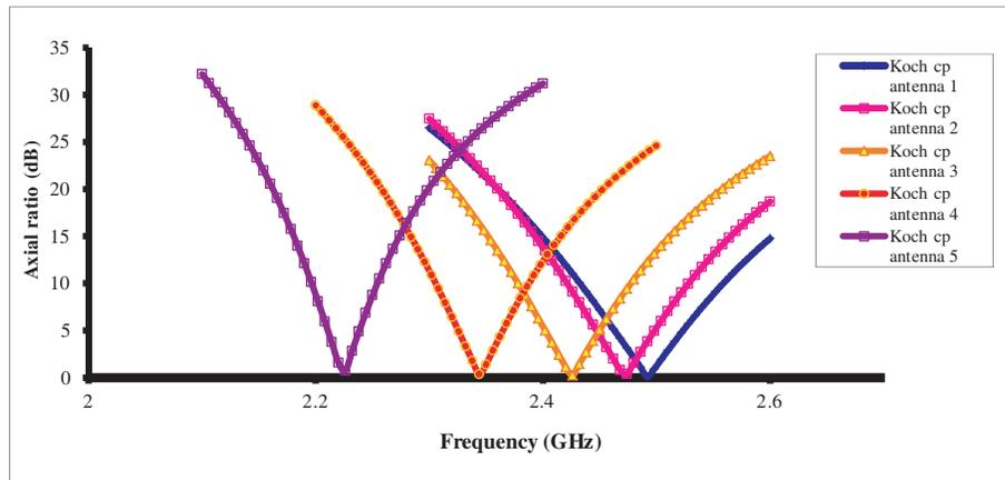
**Figure 5.** Axial ratio vs frequency of Koch fractal boundary cp antenna stage-1 for different indentation angles.
