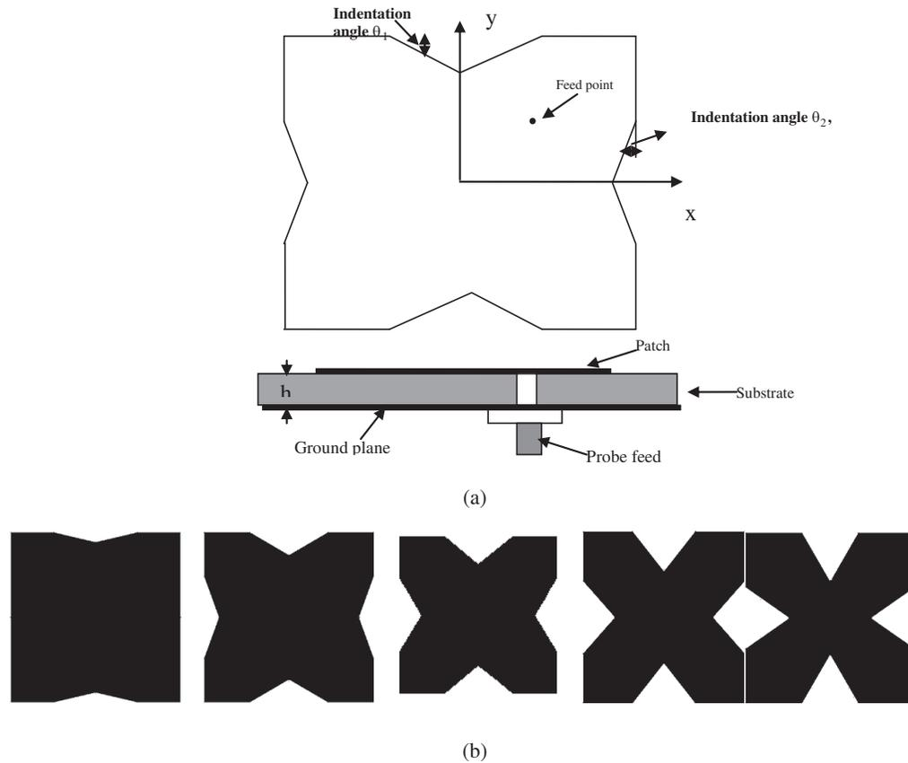
**Figure 2.** (a) Feed structure for Koch fractal boundary CP antenna. (b) Geometry of Koch CP antenna stage-1. (i)  $13^{\circ}-0^{\circ}$ , (ii)  $30^{\circ}-20^{\circ}$ , (iii)  $40^{\circ}-31^{\circ}$ , (iv)  $50^{\circ}-43^{\circ}$ , (v)  $60^{\circ}-55^{\circ}$ .
