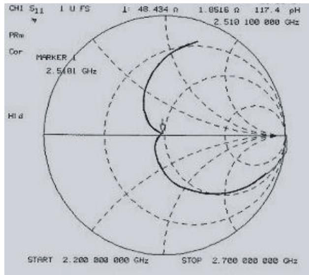
**Figure 7.** Measured input impedance of Koch CP antenna stage-1.
