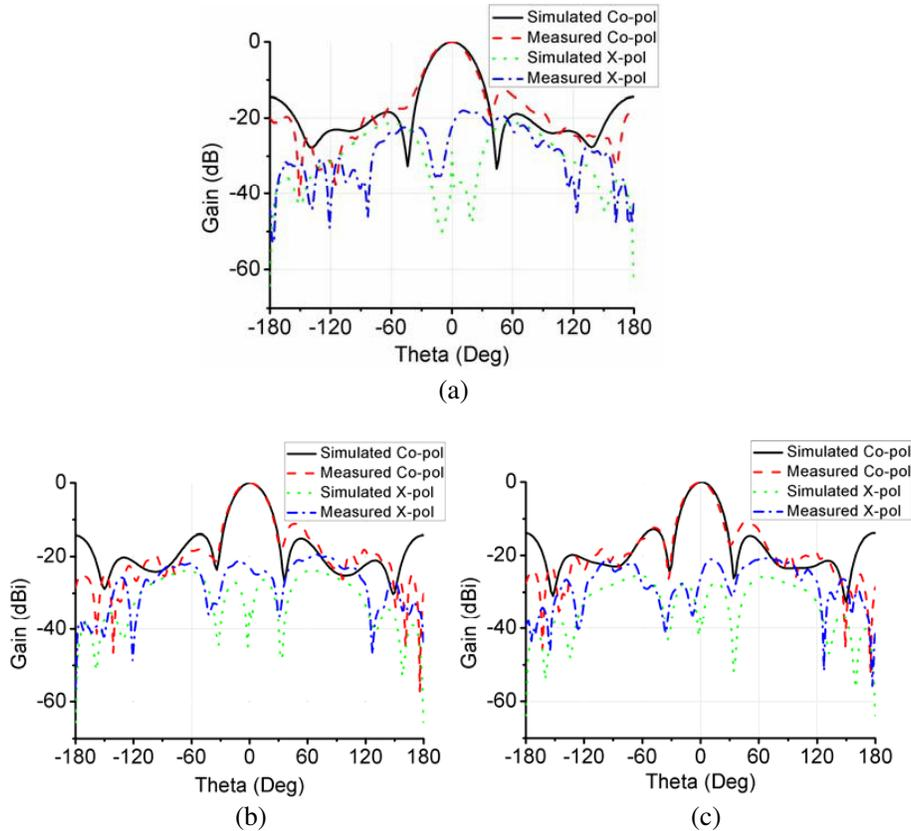
**Figure 8.** Simulated and measured radiation patterns of the array. (a)  $E$ -plane at 1.7 GHz. (b)  $E$ -plane at 1.9 GHz. (c)  $E$ -plane at 2.2 GHz.
