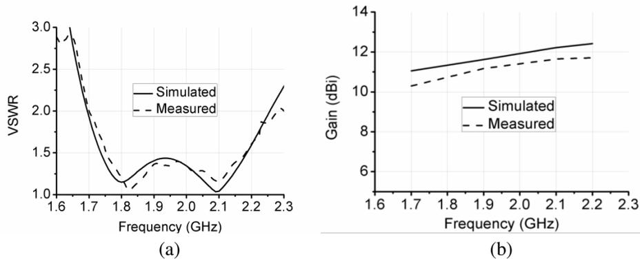
**Figure 7.** Simulated and measured results of the array. (a) VSWR, (b) gain.
