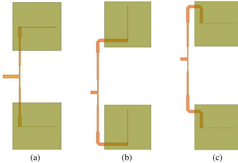
**Figure 2.** Various feed structure design of the array antenna. (a) Ant. 1 (proposed), (b) Ant. 2, (c) Ant. 3.
