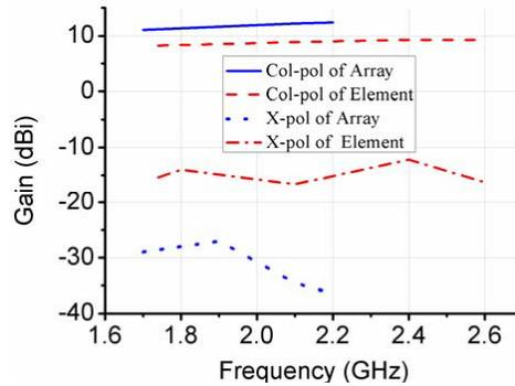
**Figure 4.** The co-polarization and cross polarization at the broadside direction in the  $E$ -plane of the array and element.
