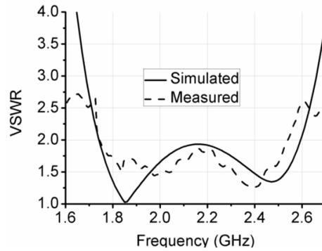
**Figure 6.** Simulated and measured results of VSWR against frequency of the element.
