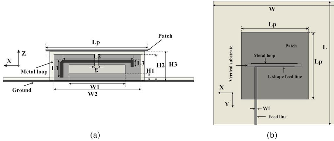
**Figure 1.** The structure and detailed dimensions of the antenna element. (a) Side view. (b) Top view.
