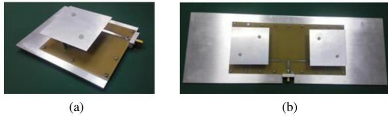
**Figure 5.** Photographs of the proposed antennas. (a) Element. (b) Array.
