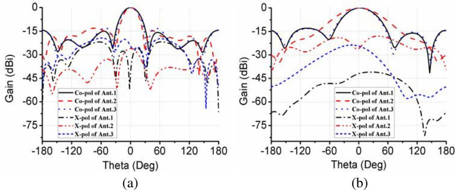
**Figure 3.** Radiation patterns of various antenna designs. (a)  $xz$ -plane at 2 GHz. (b)  $yz$ -plane at 2 GHz.
