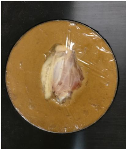
**Figure 9.** The OUT constructed from peanut butter and jam (PBJ), an absorber sheet, and a chicken wing. Note that the skin of the chicken wing has been pulled to the left side of the wing. There are also two bones inside the chicken wing that run down the center underneath the muscle tissue.
