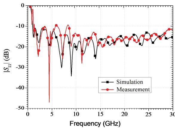
**Figure 7.** Measured and simulated return loss of the proposed cone antenna.
