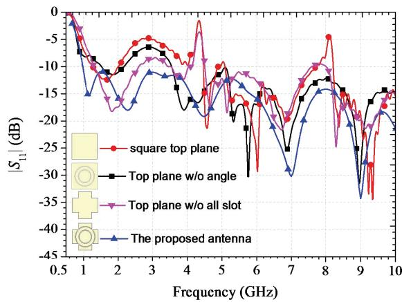
**Figure 2.** Simulated return loss of the proposed antenna with various situation of the top plane.
