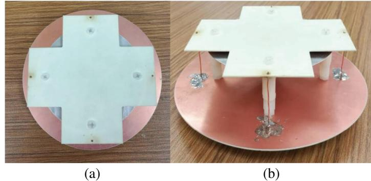
**Figure 6.** The photograph of the UWB antenna. (a) Top view. (b) Perspective view.
