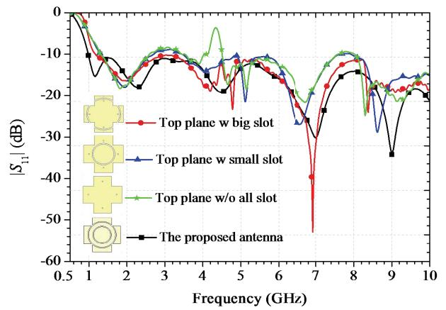
**Figure 3.** Simulated return loss of the proposed cone antenna with various slot of top plane.
