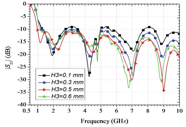
**Figure 5.** Simulated return loss of the proposed cone antenna with different spacing ( $H_3$ ) between cone and ground.
