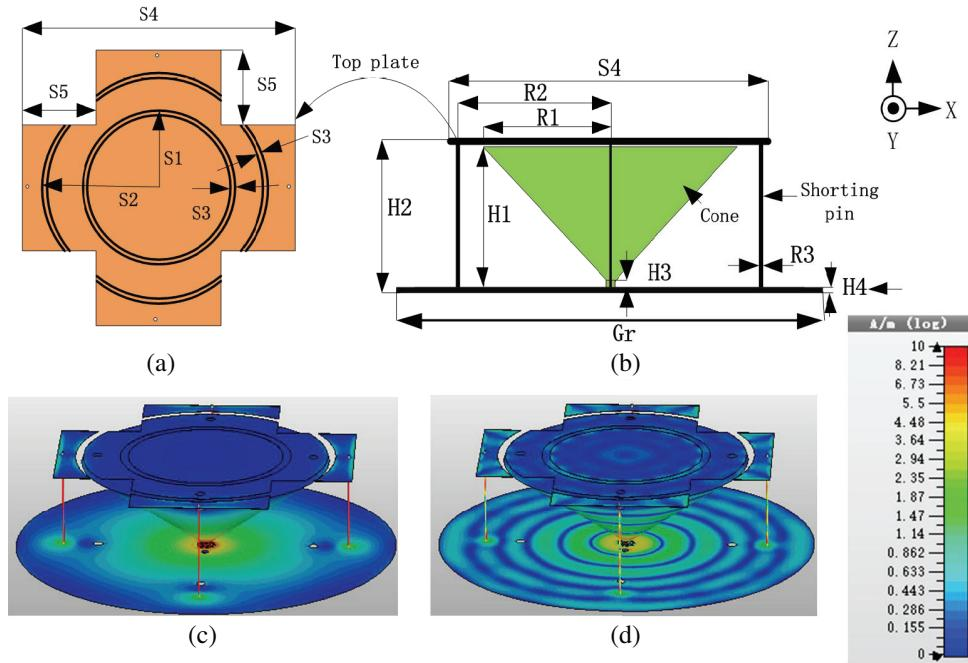
**Figure 1.** Structure diagrams (a) the top plane of the proposed design. (b) The side view of the proposed cone antenna. (c) Current distribution at 2 GHz. (d) Current distribution at 15 GHz.
