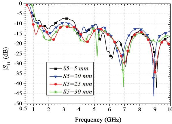
**Figure 4.** Simulated return loss of various  $S_5$  of the top-cross plane.
