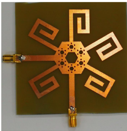
Figure 3. Fabricated hexagonal fractal navigation antenna.
