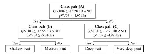
Figure 2. The classification rules and the decision tree (DT) algorithm diagram developed in this study.
