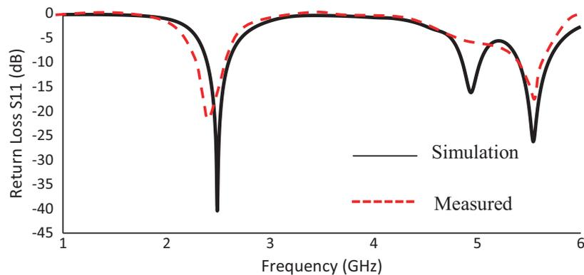
Figure 5. Return loss of proposed electrically small antenna.
