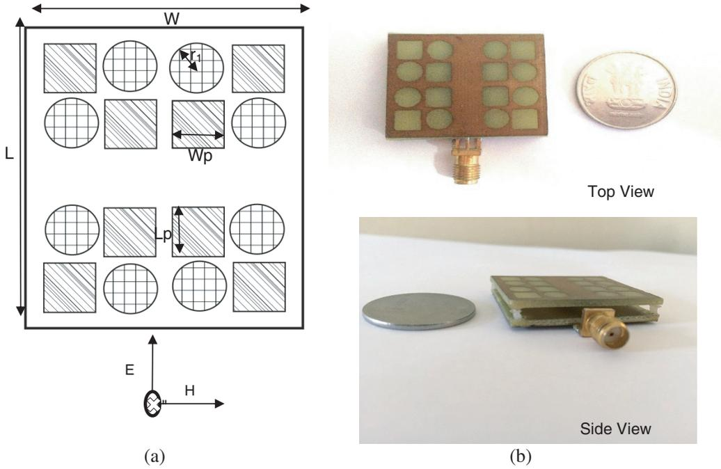
**Figure 1.** Model of the proposed antenna. (a) Geometry. (b) Fabrication of the prototype antenna.
