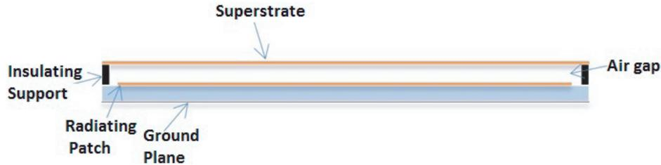
Figure 2. Layered antenna structure.
