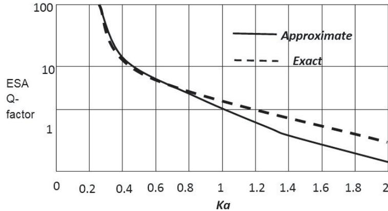
**Figure 3.** ESA  $Q$  factor vs  $ka$  curve for electrically small antenna.
