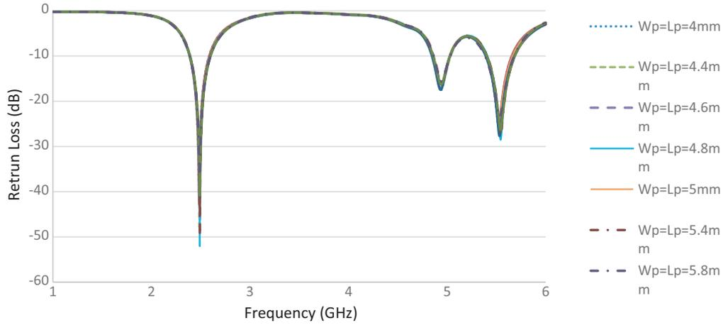
**Figure 6.** Return loss different values of  $W_p$  and  $L_p$ .
