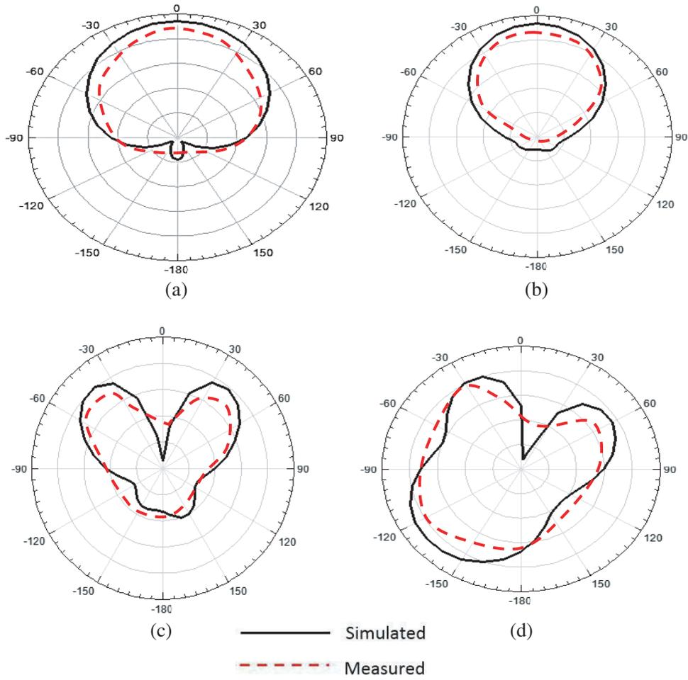
**Figure 11.** Simulated & measured radiation patterns. (a) *E*-plane at 2.4 GHz. (b) *H*-plane 2.4 GHz. (c) *E*-plane at 5.5 GHz. (d) *H*-plane 5.5 GHz.
