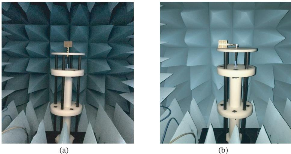
Figure 10. Anechoic chamber for radiation measurement. (a) *E*-plane. (b) *H*-plane.
