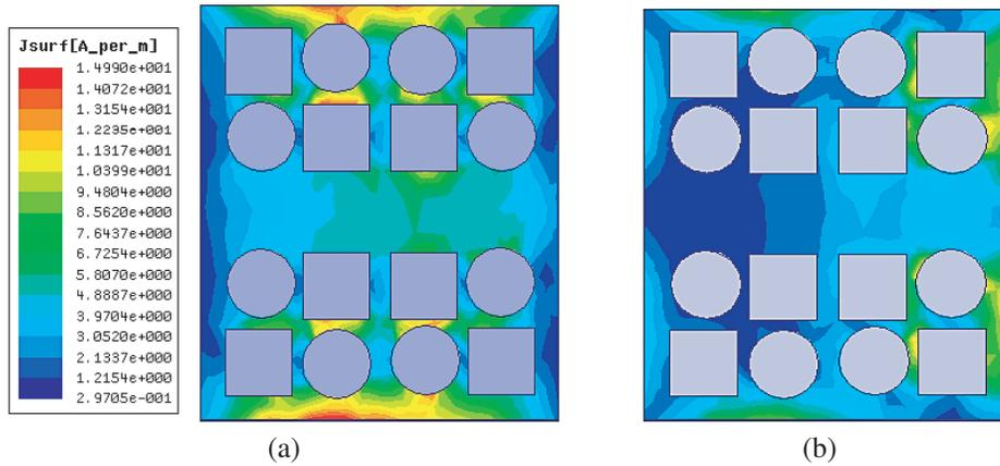
Figure 9. An electrically small antenna surface current distribution at (a) 2.4 GHz, (b) 5.5 GHz.
