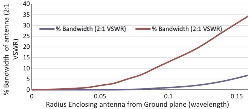
Figure 4. Fundamental limit of impedance bandwidth of small antenna.
