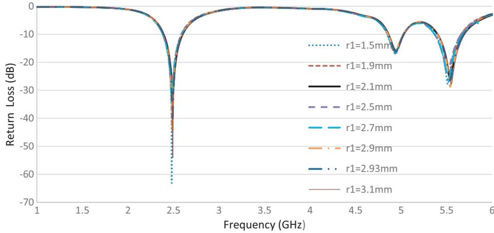
**Figure 7.** Return loss different values of  $r_1$ .
