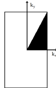
Figure 5. The First Brillouin Zone of the metal photonic crystal with the rectangular lattice.
