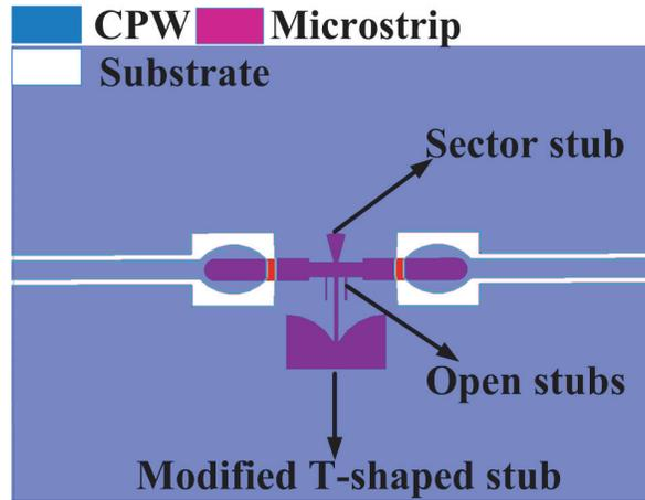
**Figure 1.** Configuration of the proposed UWB BPF.
