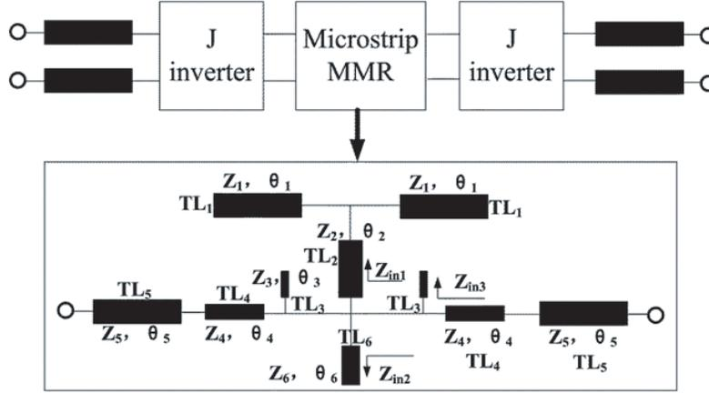
Figure 2. Equivalent J-inverter network of the proposed filter.
