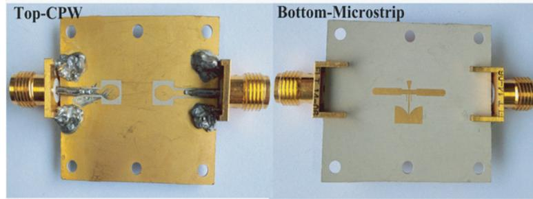
**Figure 4.** Photograph of the fabricated UWB BPF.
