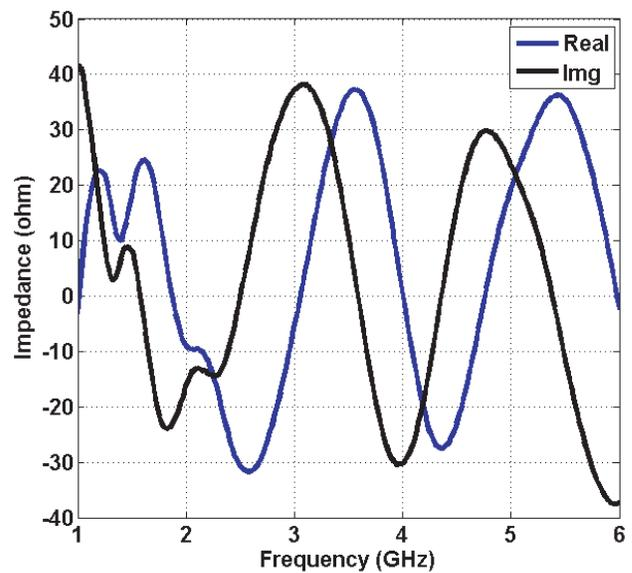
Figure 4. Measured input impedance of antenna 1.
