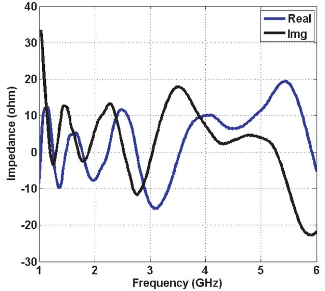
**Figure 6.** Measured input impedance of antenna 2.
