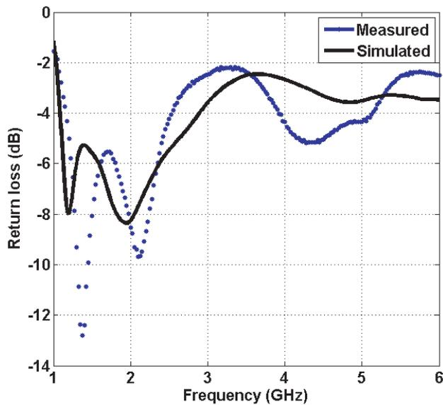
Figure 3. Measured and simulated return loss antenna 1.
