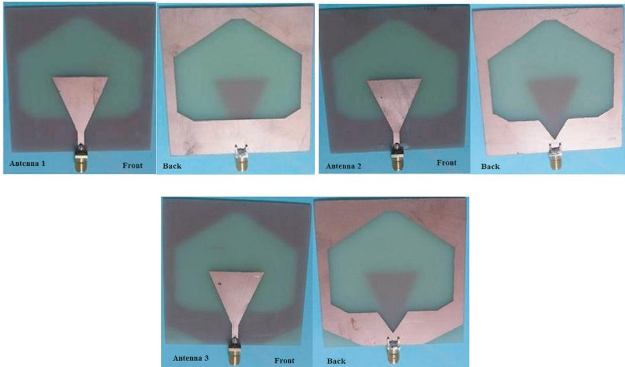
Figure 2. Prototypes of antenna 1, 2 and 3.
