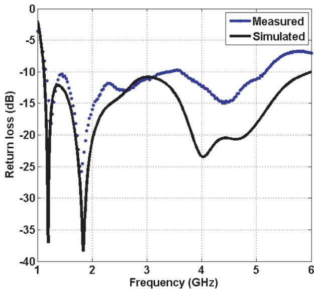
**Figure 7.** Measured and simulated return loss antenna 3.
