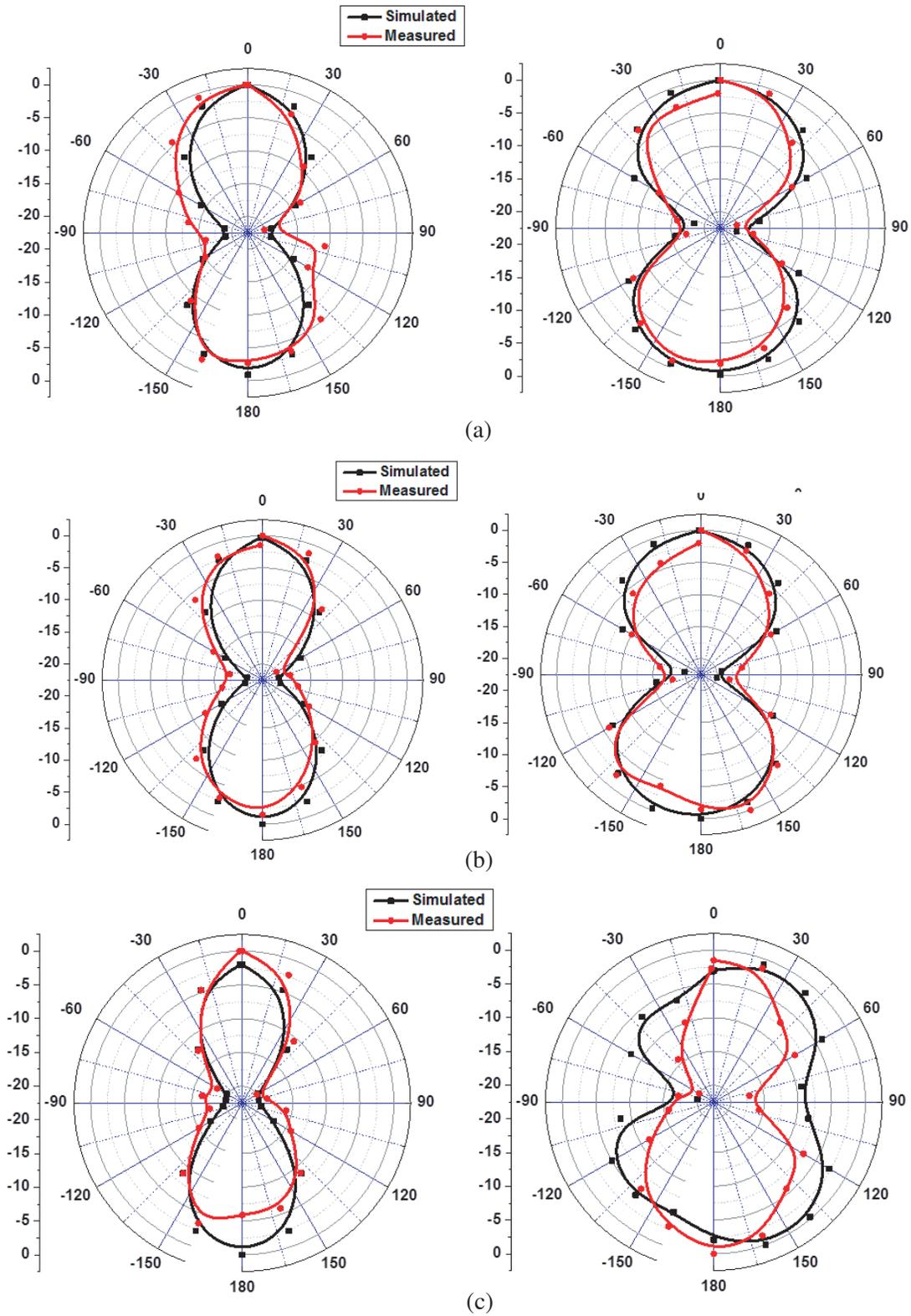
Figure 10. Far field patterns ( $E$ -plane (left),  $H$ -plane (right)) at frequencies (a) 1.25 GHz, (b) 1.9 GHz and (c) 4.2 GHz.
