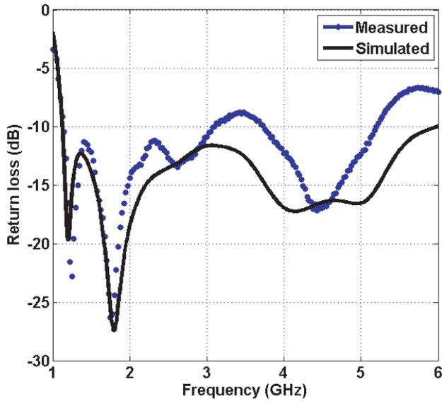
**Figure 5.** Measured and simulated return loss antenna 2.
