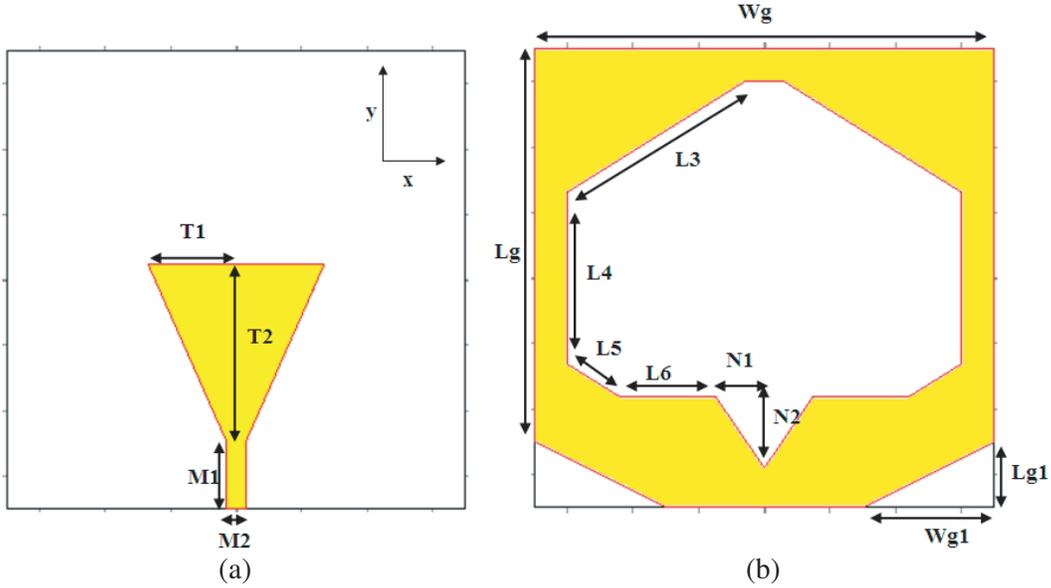
**Figure 1.** Geometry of proposed antenna. (a) Top view, (b) bottom view (yellow colour is metal).
