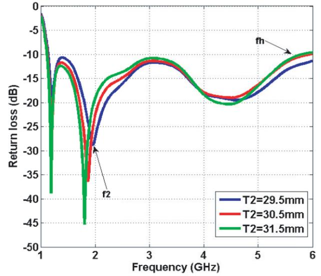
**Figure 12.** Effect of  $T2$  on the frequency response of the antenna.
