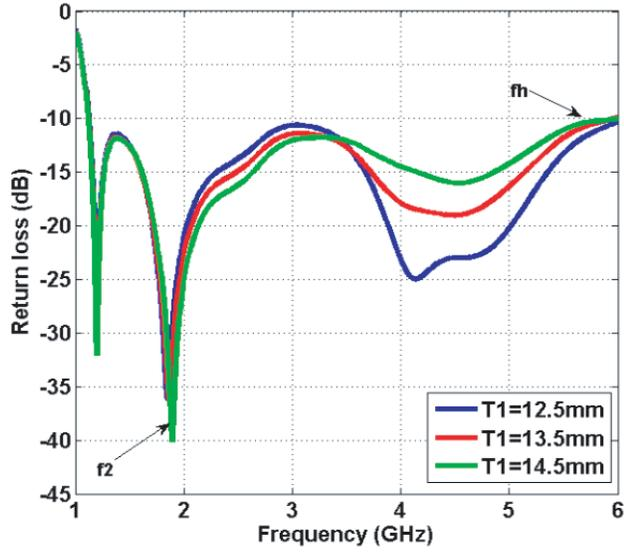
**Figure 11.** Effect of  $T1$  on the frequency response of the antenna.
