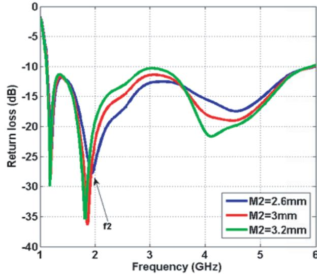
**Figure 13.** Effect of  $M2$  on the frequency response of the antenna.
