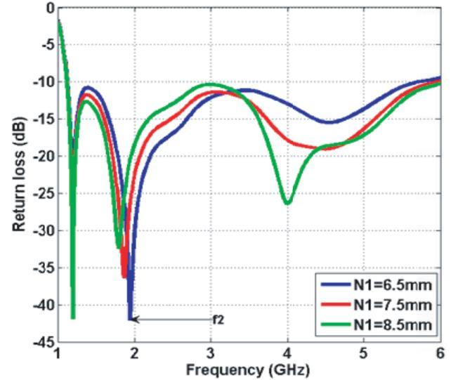
**Figure 14.** Effect of  $N1$  on the frequency response of the antenna.
