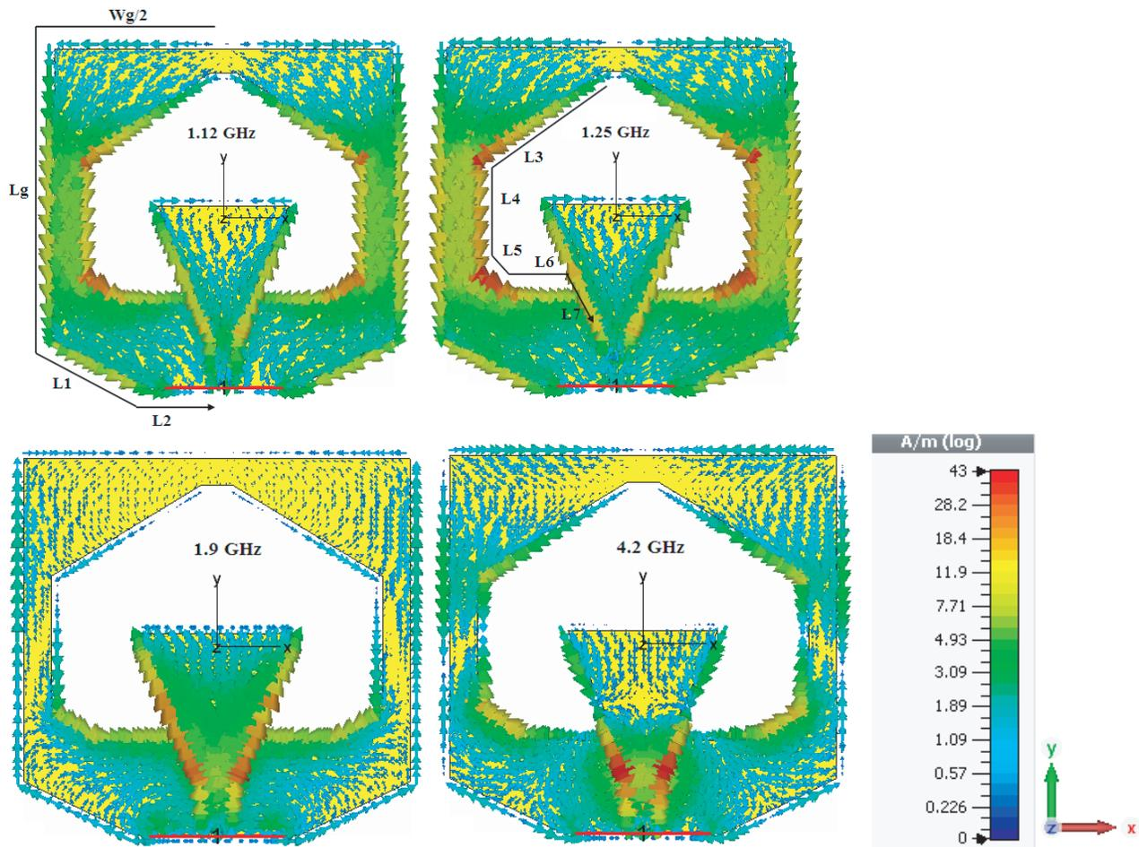
**Figure 9.** Surface current distributions of proposed antenna at the lower cut-off frequency and resonating frequencies.
