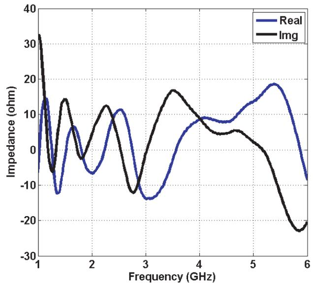
**Figure 8.** Measured input impedance of antenna 3.
