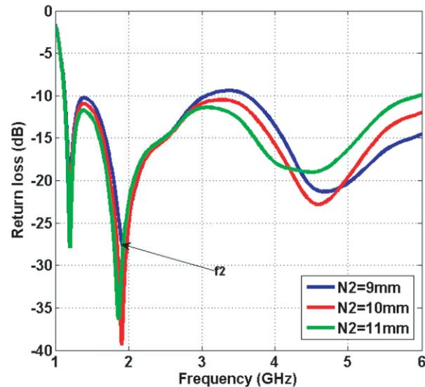
**Figure 15.** Effect of  $N2$  on the frequency response of the antenna.
