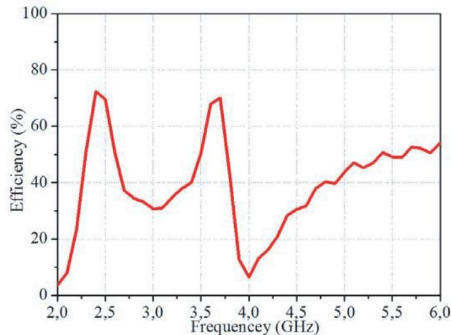
**Figure 10.** Radiation efficiency of the proposed antenna.
