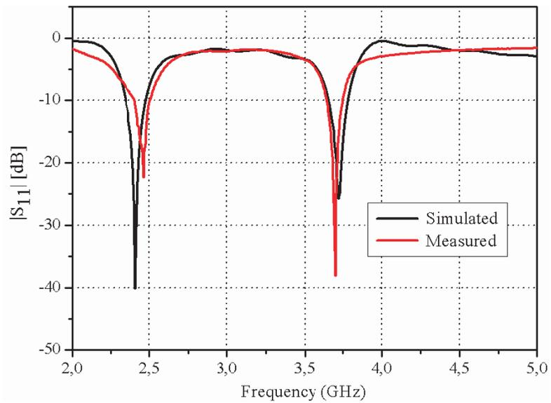
**Figure 8.** Measured and simulated reflection coefficients of the proposed antenna.
