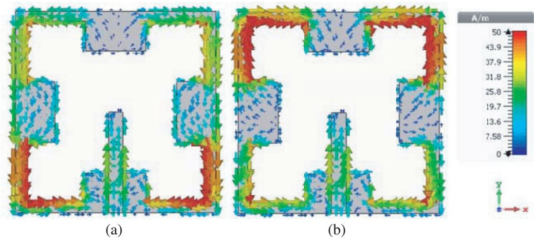
**Figure 6.** Simulated surface current distribution observed from the ground planeside: (a) 2.4 and (b) 3.75 GHz.
