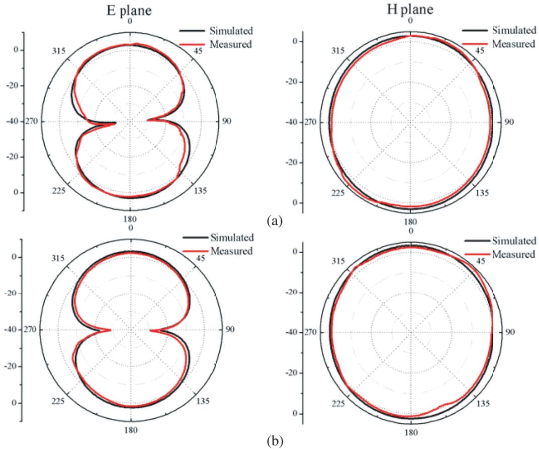
**Figure 9.** Measured and simulated radiation patterns of the proposed antenna in the  $H$ - and  $E$ -planes at (a) 2.4 GHz, (b) 3.75 GHz.
