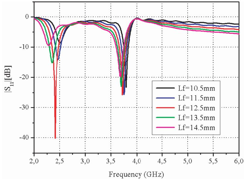
**Figure 5.** Effect of the feed line length  $L_f$  on the reflection coefficient.
