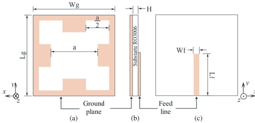
**Figure 1.** Configuration of the proposed antenna. (a) Bottom. (b) Side. (c) Top.
