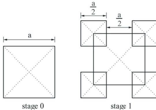
**Figure 2.** Iterations of the proposed fractal antenna.
