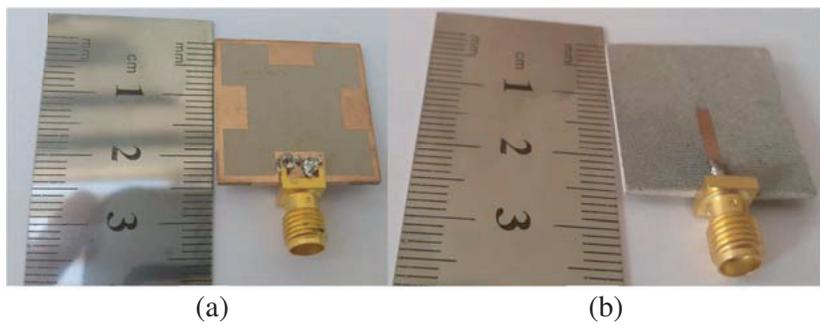
**Figure 7.** Photograph of the fabricated antenna. (a) Bottom. (b) Top.
