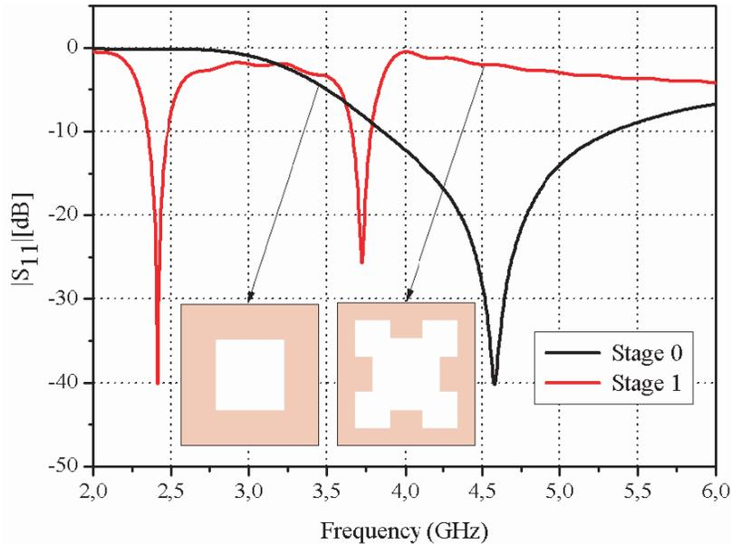
**Figure 3.** Simulated reflection coefficients for the two proposed stages.
