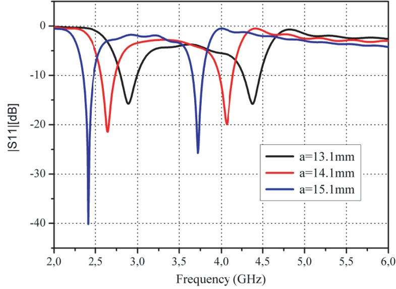
**Figure 4.** Effect of the grounded slot length  $a$  on the reflection coefficient.
