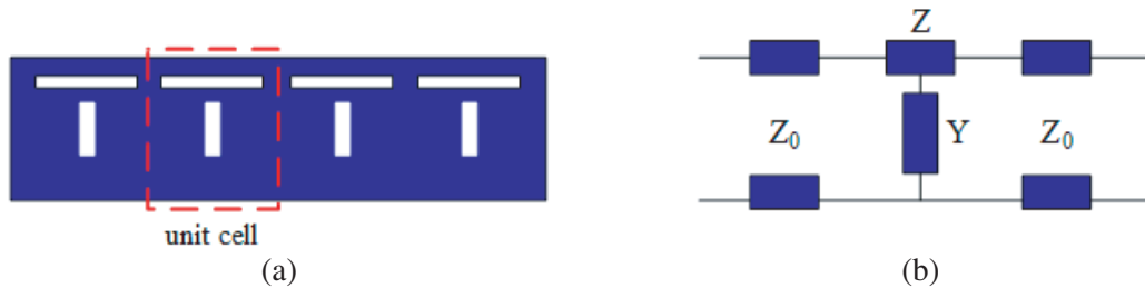
Figure 1. Periodic slots located on the broad wall of a rectangular waveguide, (a) periodic unit cell structure; (b) the equivalent circuit of the unit cell.
