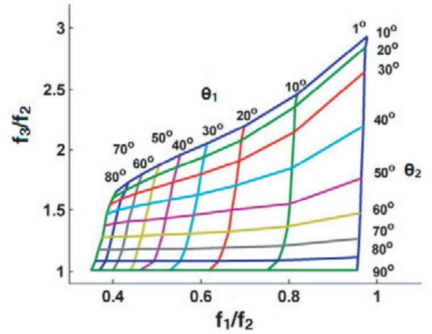
**Figure 2.** Design curve for crossed resonator.
