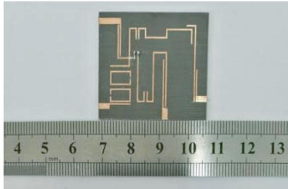
**Figure 9.** Photograph of the fabricated triplexer.
