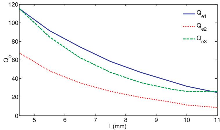
Figure 5. Extracted external quality factors at different frequencies.
