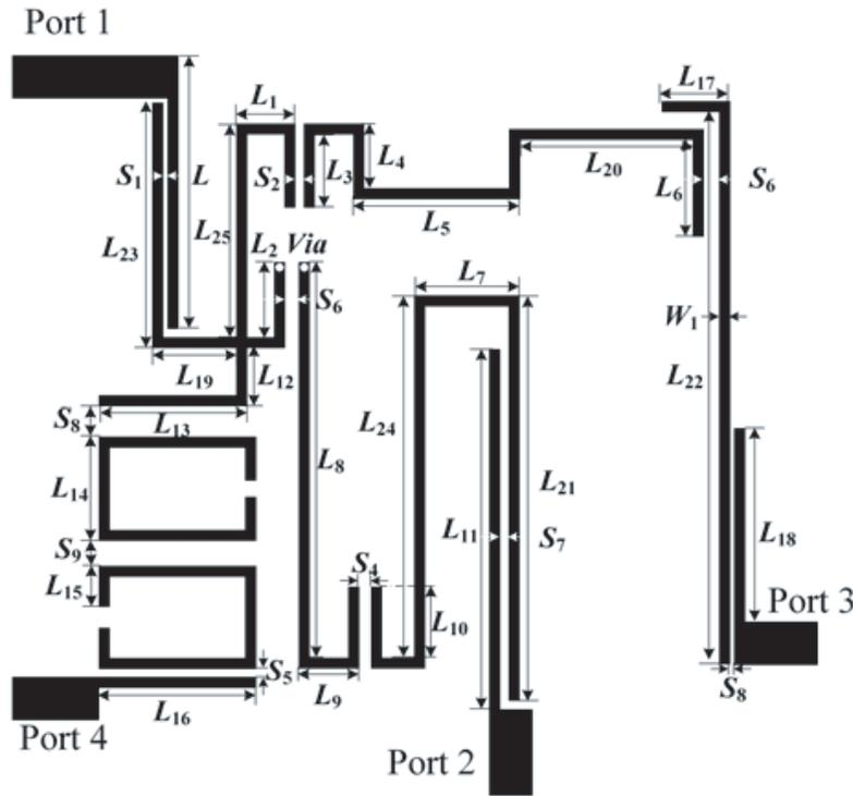
**Figure 3.** Layout of the triplexer using crossed resonator.
