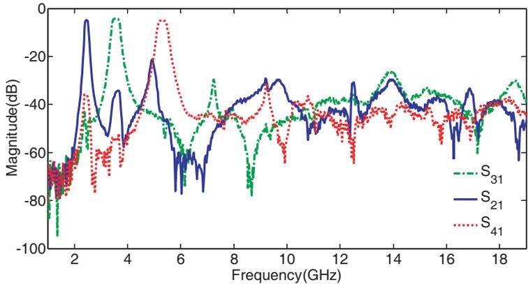
**Figure 8.** Measured wideband response of the triplexer.
