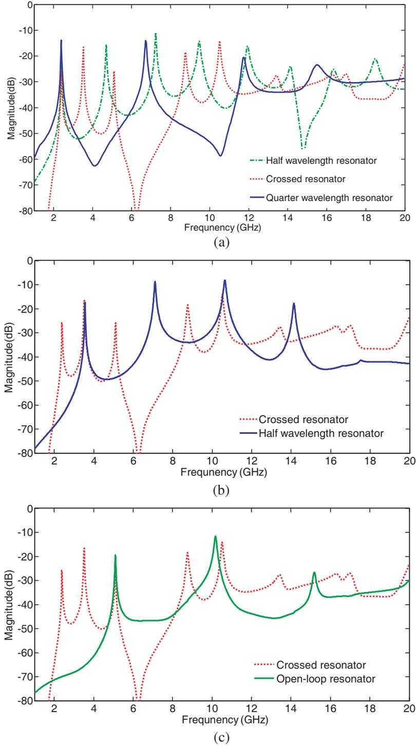
**Figure 4.**  $S$  parameters of test resonators in different channel filters contrasting to the crossed resonator. (a) The first channel. (b) The second channel. (c) The third channel.
