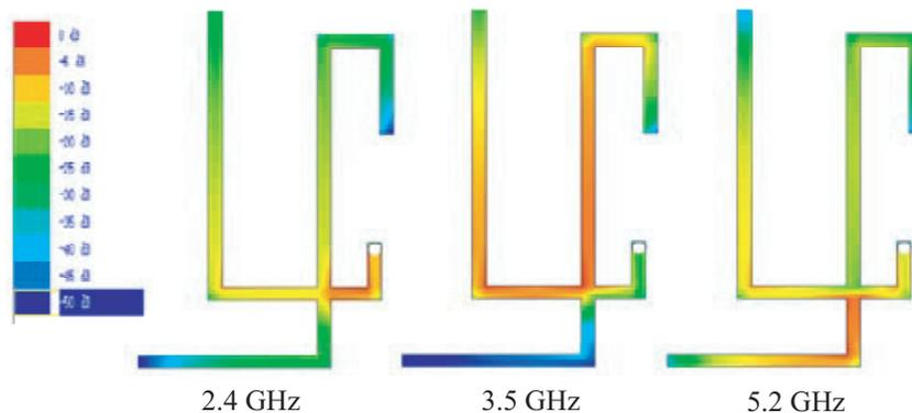
Figure 6. Current distribution at the first three resonance frequencies of the crossed resonator.
