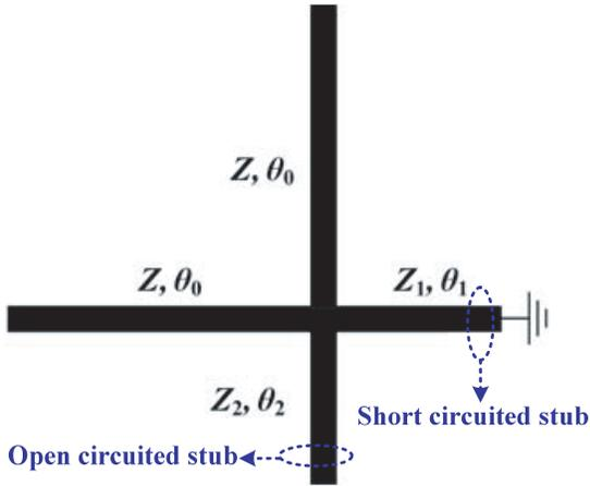
**Figure 1.** Structure of the proposed crossed resonator.
