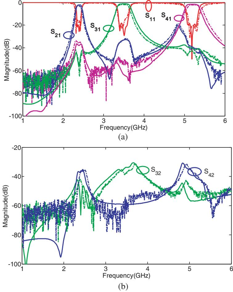
**Figure 7.** Simulated (solid line) and measured (dash line)  $S$  parameters of the triplexer. (a)  $S_{11}, S_{21}, S_{31}, S_{41}$ . (b) Isolations of the triplexer.
