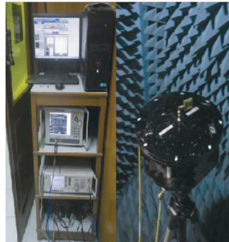
Figure 13. Experimental setup for measurement of radiation patterns in an anechoic chamber.
