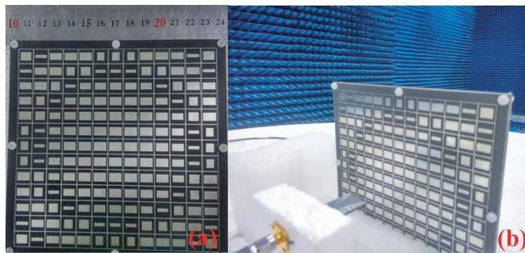
**Figure 17.** Photographs of the (a) proposed MS and (b) its measured surroundings.
