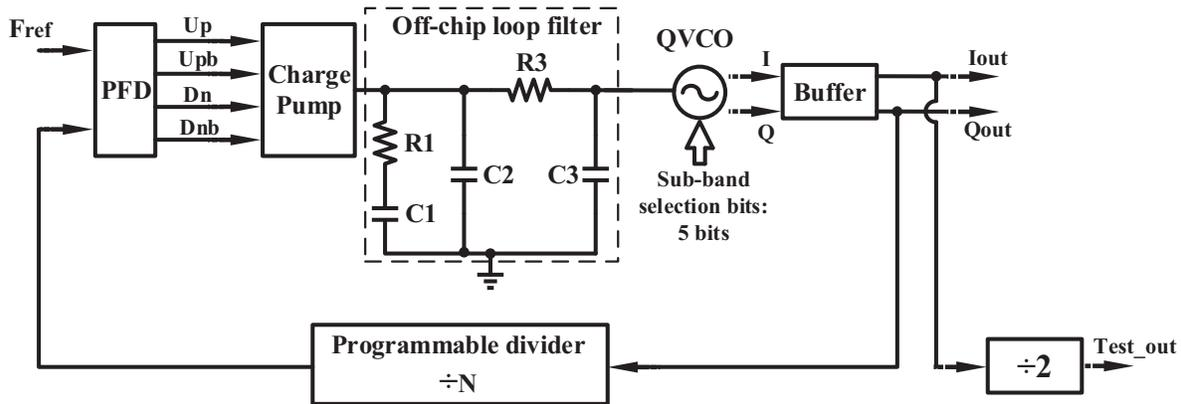
**Figure 1.** Block diagram of frequency synthesizer.
