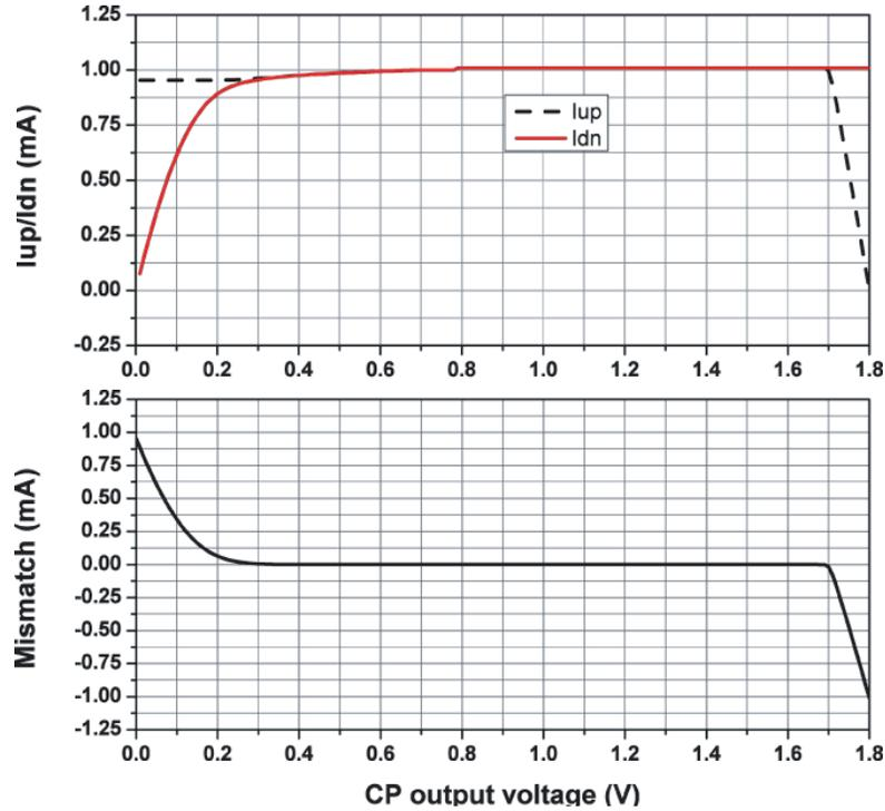
**Figure 4.** Simulated up/down currents and mismatch between up/down currents versus CP output voltage.
