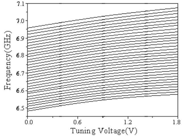
**Figure 13.** Measured frequency tuning characteristic of bottom-series QVCO.
