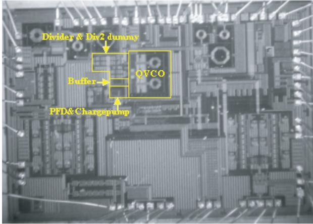
**Figure 12.** Chip photograph of frequency synthesizer integrated in a UWB transceiver.
