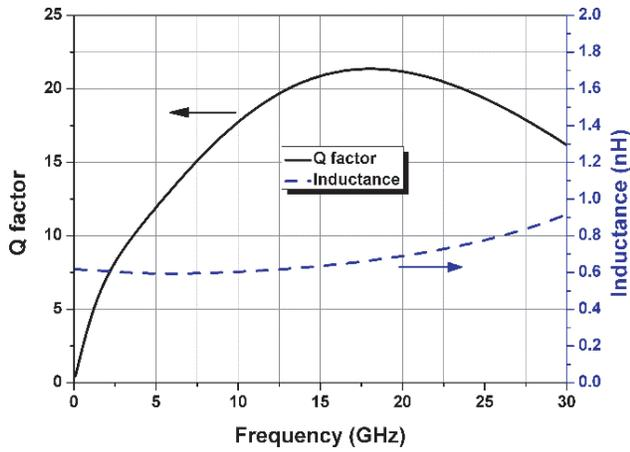
**Figure 9.** Inductor  $Q$ -factor and inductance versus frequency.
