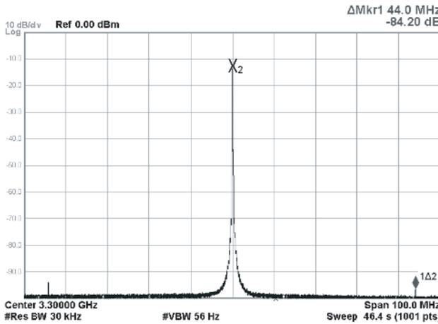
**Figure 14.** Measured 3.3 GHz frequency spectrum of the synthesizer locked in 6.6 GHz.
