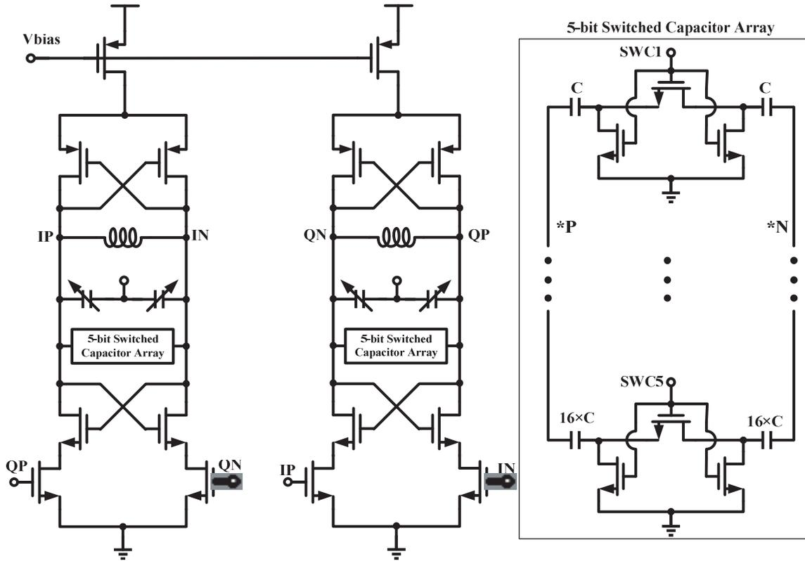
Figure 8. Schematic of the bottom-series QVCO.
