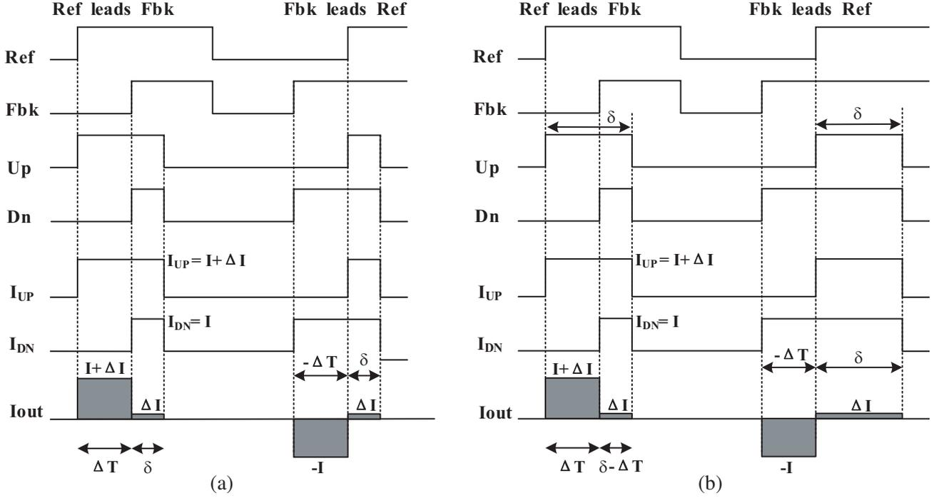
**Figure 6.** Timing diagram for PFD and CP: (a) traditional delay scheme, (b) new delay scheme.
