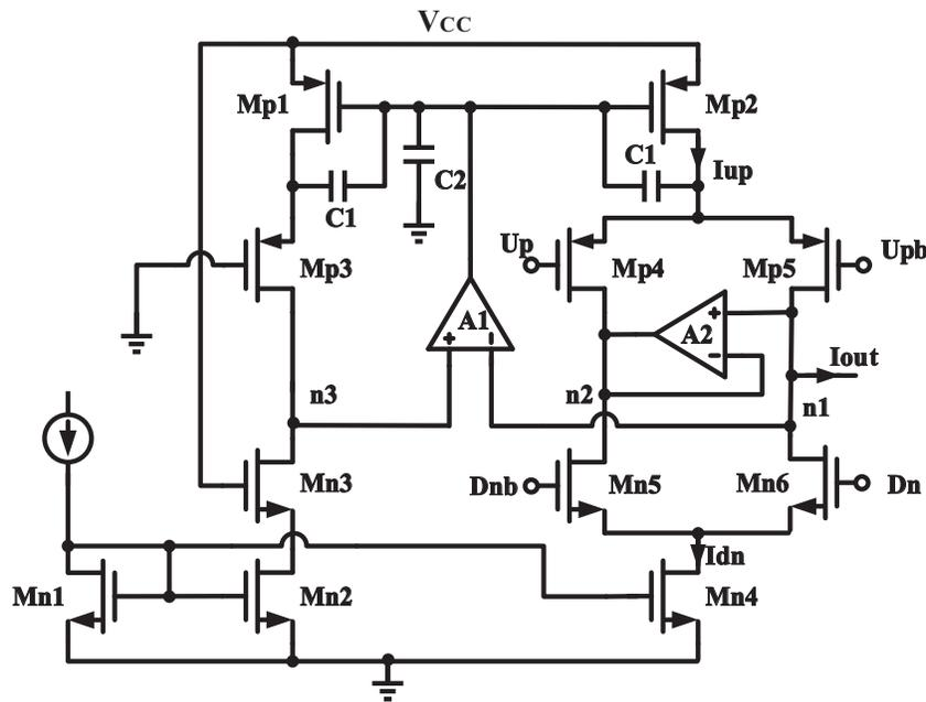
Figure 3. Schematic of the charge pump circuit.
