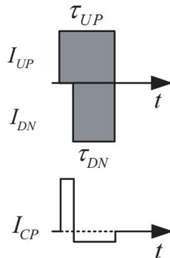
**Figure 2.** Charge pump output current in locked state due to current mismatch.
