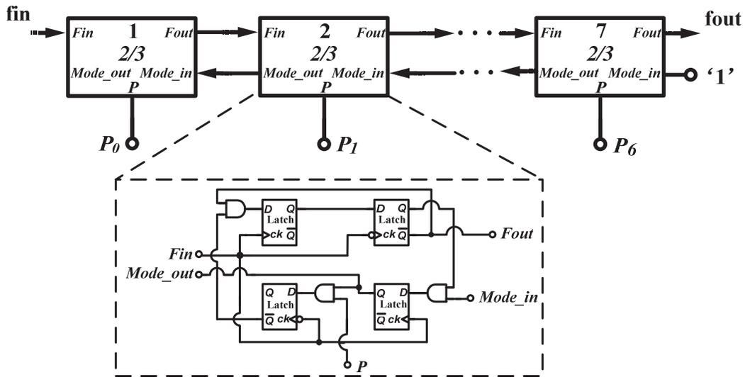
**Figure 11.** Schematic of the programmable multi-modulus divider.
