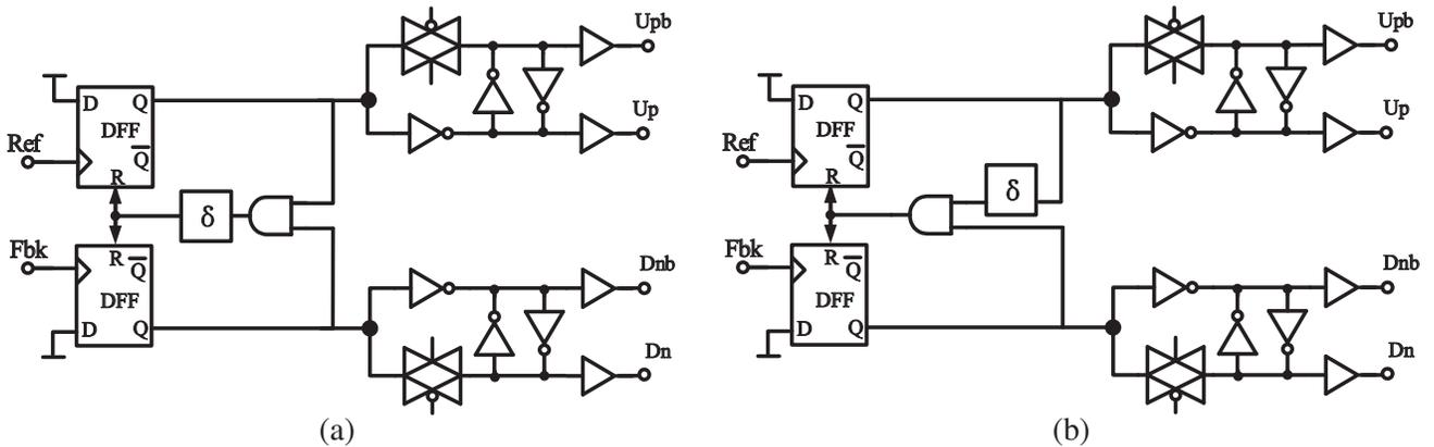
**Figure 5.** (a) Schematic of the traditional PFD, (b) schematic of the highly linear PFD used in this work.
