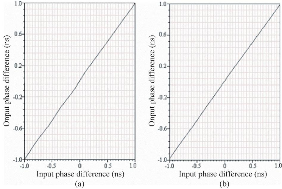
**Figure 7.** Simulated transfer-function curves of PFD and CP: (a) traditional delay scheme, (b) new delay scheme.
