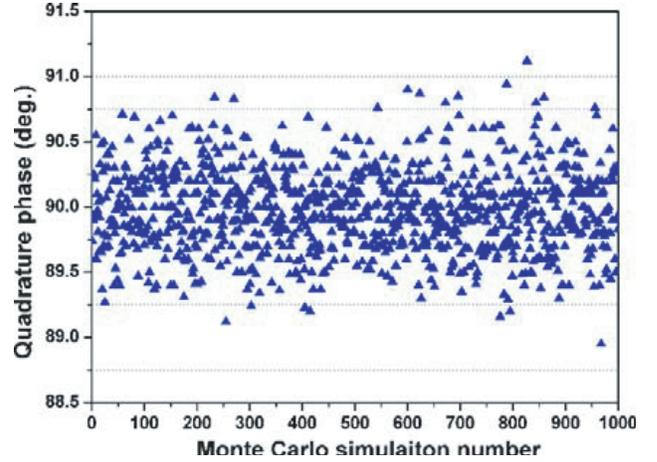
**Figure 10.** Effect of capacitor and transistor mismatches on QVCO quadrature phase based on Monte Carlo simulation.
