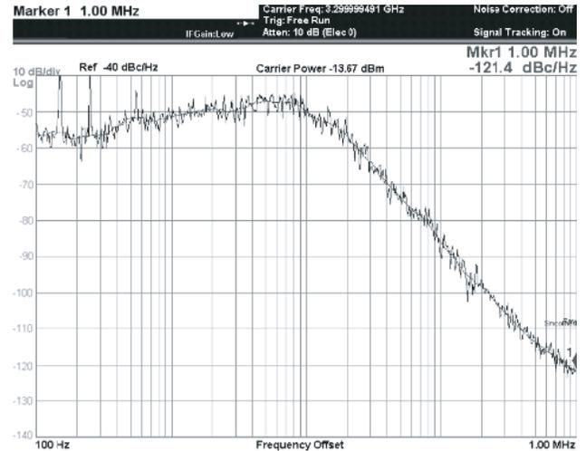
**Figure 15.** Measured 3.3 GHz close-loop phase noise of the synthesizer locked in 6.6 GHz.
