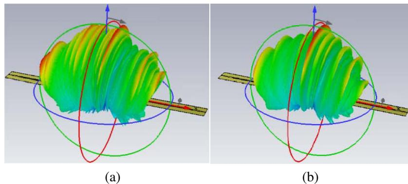
**Figure 4.** 3D far-field of the aperture at the frequency of (a) 33 GHz and (b) 37 GHz.
