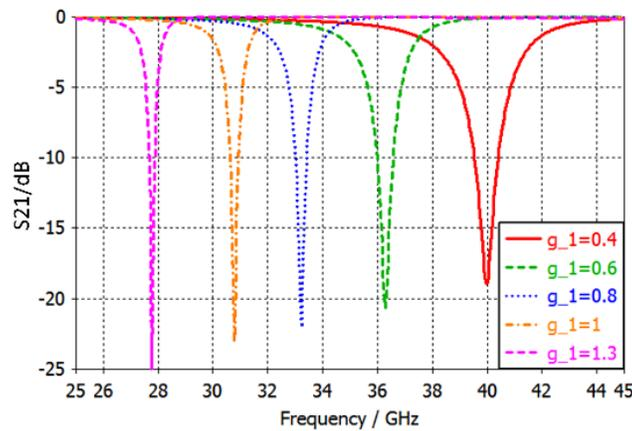
**Figure 3.** The resonance frequency of cELC unit with different length of  $g$ .
