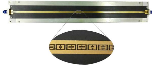
Figure 5. Photograph of fabricated metamaterial aperture.
