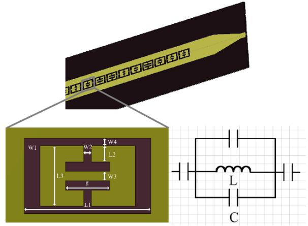
**Figure 2.** The structure of metamaterial aperture and equivalent circuit model of cELC unit.
