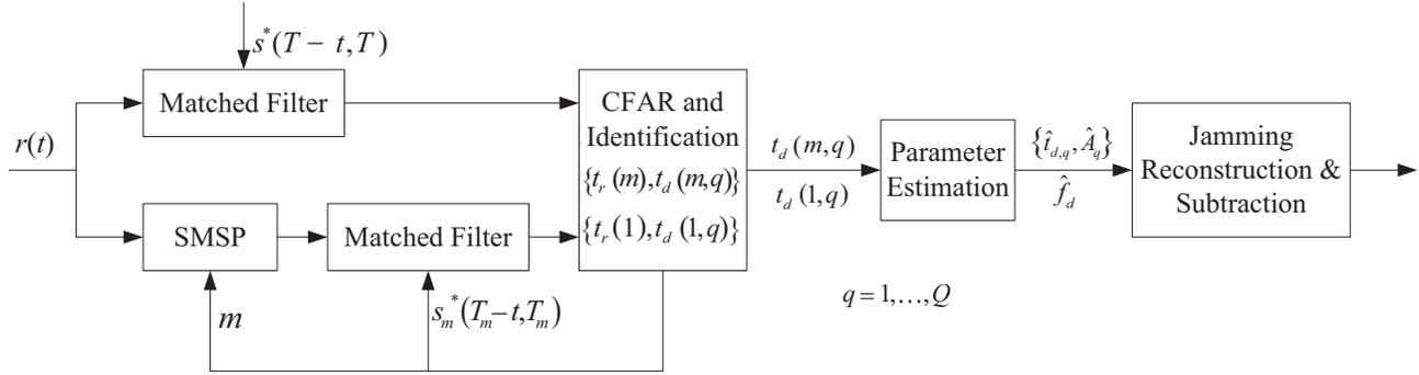
**Figure 3.** Smart noise jamming suppression scheme.
