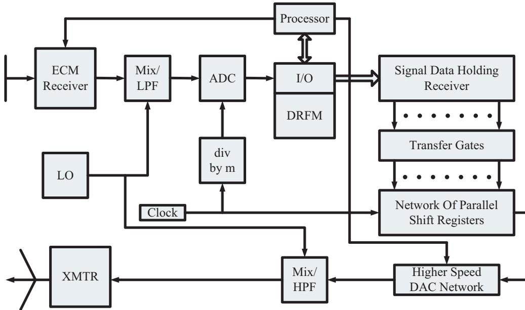
**Figure 2.** The block diagram of SMSP jamming generator.
