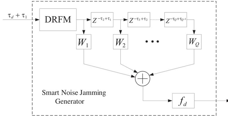
**Figure 1.** The block diagram of smart noise jamming generator.
