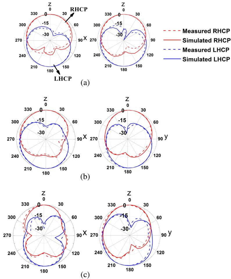
**Figure 9.** Simulated and measured radiation patterns in  $x$ - $z$  plane and  $y$ - $z$  plane at (a) 2.6 GHz, (b) 3.5 GHz, (c) 4.4 GHz.
