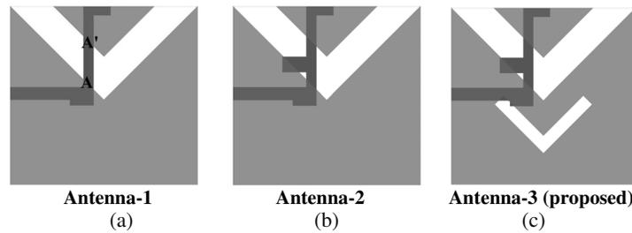
Figure 3. Antenna design process from Antenna-1 (a) to Antenna-3 (c).
