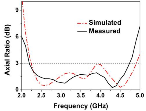
**Figure 6.** Simulated and measured results of axial ratio.
