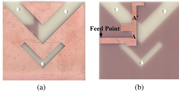
**Figure 2.** Prototype of the proposed antenna, (a) top view, (b) bottom view.
