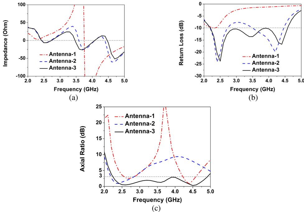
Figure 4. Simulated (a) impedance imaginary part, (b) return loss and (c) AR for Antenna-1, 2, and 3.
