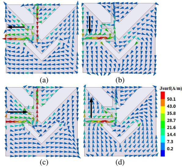
**Figure 8.** Simulated surface current distributions of the antenna at 2.8 GHz, (a)  $0^\circ$ , (b)  $90^\circ$ , (c)  $180^\circ$ , (d)  $270^\circ$ .
