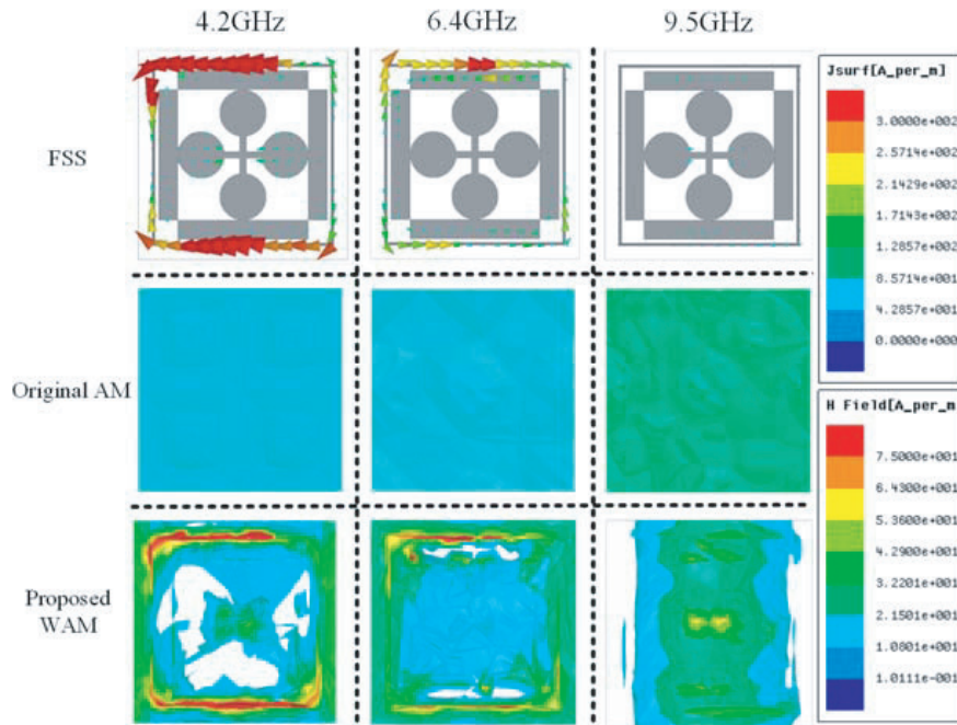
Figure 3. Vector plot of the surface current density in FSS and magnetic fields in two AMs at 4.2, 6.4, and 9.5 GHz.
