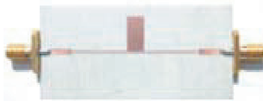
Figure 10. Photograph of fabricated Hi-Lo low-pass filter using stub capacitor.
