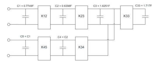
Figure 2. Inverter-coupled DBLPP configuration.
