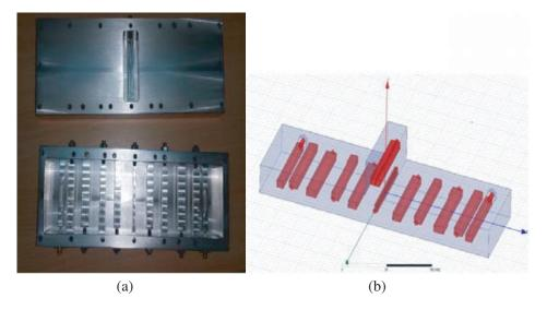
Figure 7. (a) Modified DBBPF interdigital filter prototype; (b) 3D HFSS DBBPF model.
