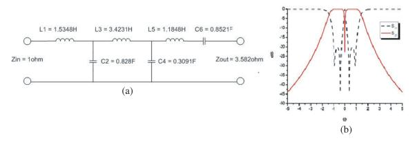
Figure 6. (a) Ladder network DBLLP configuration; (b) Simulated DBLLP response.
