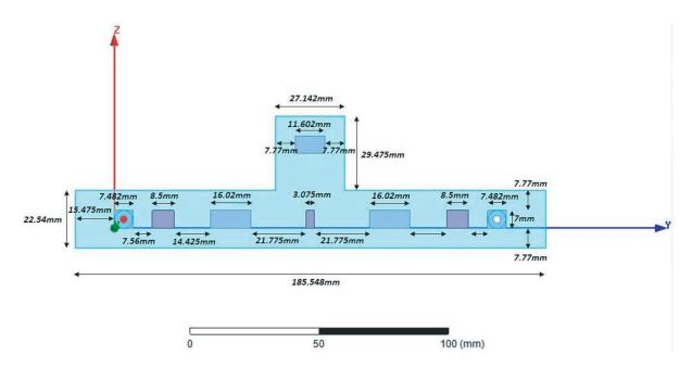
Figure 4. 2D HFSS DBBPF with measurements.
