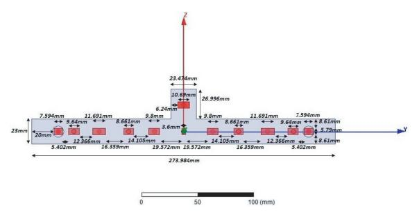
Figure 8. 2D HFSS model with measurements.
