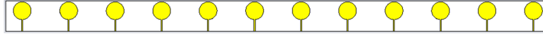
Figure 7. Synthesized Chebyshev array using M = 12 elements with uniform element spacing d_o = 0.835 \lambda = 125.25 mm at f = 1.5 GHz.
