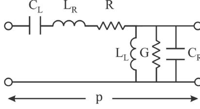
**Figure 1.** Equivalent circuit model of a general CRLH unit cell.
