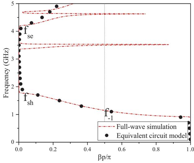
**Figure 3.** Dispersion diagram of the proposed CRLH unit cell. The extracted circuit parameters are:  $C_L = 0.35$  pF,  $C_R = 0.52$  pF,  $L_L = 15.4$  nH,  $L_R = 4.1$  nH,  $G = 0.3$  mS and  $R = 2$   $\Omega$ .
