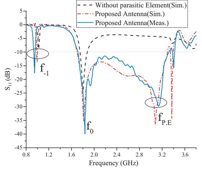
**Figure 4.** Simulated and measured reflection coefficients of the proposed antenna.
