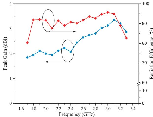
**Figure 8.** Measured gain and radiation efficiency of the proposed antenna.
