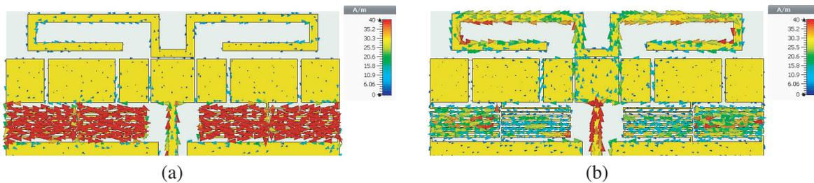
**Figure 6.** Simulation results of surface current distribution at (a)  $f = 1.84$  GHz and (b)  $f = 3.1$  GHz obtained from CST software.
