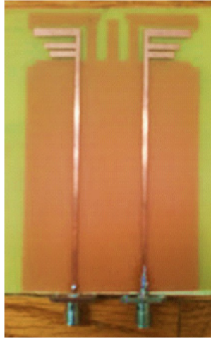
Figure 6. A photograph of the fabricated prototype MIMO antenna.
