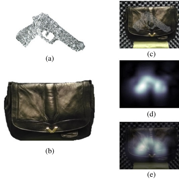
Figure 12. Holographic imaging and reconstruction at z = 0.99 m of prop gun concealed within a soft leather purse. (a) Concealed prop gun. (b) Soft leather purse. (c) Radar view of purse with concealed prop gun. (d) Reconstructed image showing concealed prop gun, and (e) Detected prop gun relative to its location of concealment.
