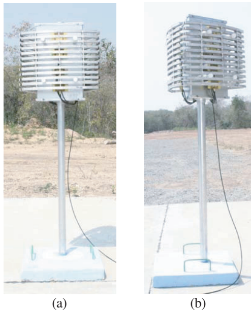
Figure 10. The prototype of the proposed triangular array antenna. (a) Front view. (b) Side view.
