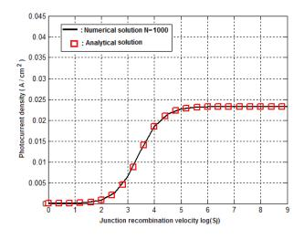
Figure 12. Photocurrent density versus Sj;  $D = 26 \text{ cm}^2/\text{s}$ ; L = 0.01 cm;  $Sb = 10^3 \text{ cm/s}$ , front surface illumination.
