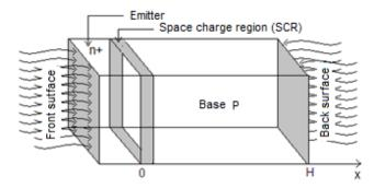
Figure 1. Silicon bifacial solar cell.
