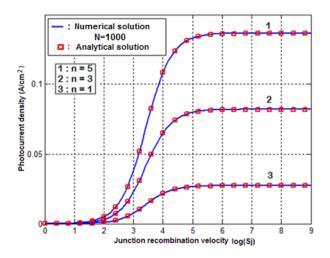
Figure 13. Photocurrent density versus Sj for various values of illumination level n:  $D = 26 \text{ cm}^2/\text{s}$ ; L = 0.01 cm;  $Sb = 10^3 \text{ cm/s}$ , front surface illumination.
