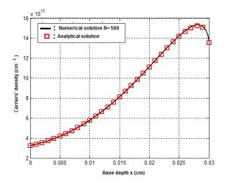
Figure 7. Minority carrier's density;  $D = 26 \text{ cm}^2/\text{s}$ ; L = 0.01 cm;  $Sb = 10^3 \text{ cm/s}$ , back surface illumination.
