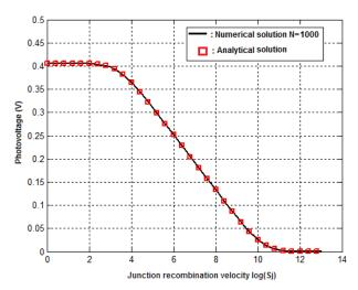
Figure 14. Photocurrent density versus Sj:  $D = 26 \text{ cm}^2/\text{s}$ ; L = 0.01 cm;  $Sb = 10^3 \text{ cm/s}$ , back surface illumination.
