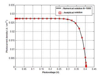
Figure 16. Current-voltage characteristics;  $D = 26 \text{ cm}^2/\text{s}$ ; L = 0.01 cm;  $Sb = 10^3 \text{ cm/s}$ , front surface illumination.
