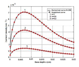
Figure 6. Minority carriers density for various back surface recombination velocities Sb:  $D = 26 \text{ cm}^2/\text{s}$ ; L = 0.01 cm;  $Sj = 10^4 \text{ cm/s}$ , front surface illumination.
