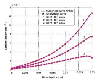
Figure 8. Minority carriers density for various back surface recombination velocities Sb:  $D = 26 \text{ cm}^2/\text{s}$ ; L = 0.01 cm;  $Sj = 10^4 \text{ cm/s}$ , back surface illumination.
