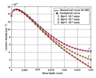
Figure 4. Minority carriers density for various junction recombination velocities Sj:  $D = 26 \text{ cm}^2/\text{s}$ ; L = 0.01 cm;  $Sb = 10^3 \text{ cm/s}$ , front surface illumination.
