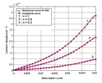
**Figure 9.** Minority carriers density for various values of n:  $D = 26 \text{ cm}^2/\text{s}$ ; L = 0.01 cm;  $Sj = 10^5 \text{ cm/s}$ ,  $Sb = 10^3 \text{ cm/s}$ , back surface illumination.
