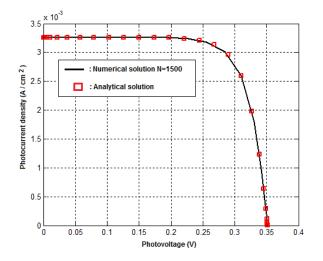
Figure 17. Current-voltage characteristics:  $D = 26 \text{ cm}^2/\text{s}$ ; L = 0.01 cm;  $Sb = 10^3 \text{ cm/s}$ , back surface illumination.
