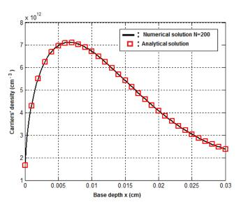
Figure 3. Minority carrier's density;  $Sj = 10^5$  cm/s: D = 26 cm<sup>2</sup>/s; L = 0.01 cm;  $Sb = 10^3$  cm/s, front surface illumination.
