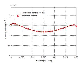
x 10<sup>13</sup> : Numerical curve N=800 2 Analytical curve Carriers' density (cm <sup>- 3</sup> ) n = 1n = 0.6 n = 0.4 0.5 0 0 0.005 0.03 0.01 0.015 0.02 0.025 Base depth x (cm)
