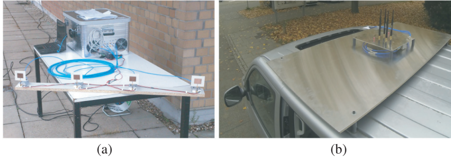
Figure 6. (a) Stationary transmitter setup and (b) mobile receiver setup.
