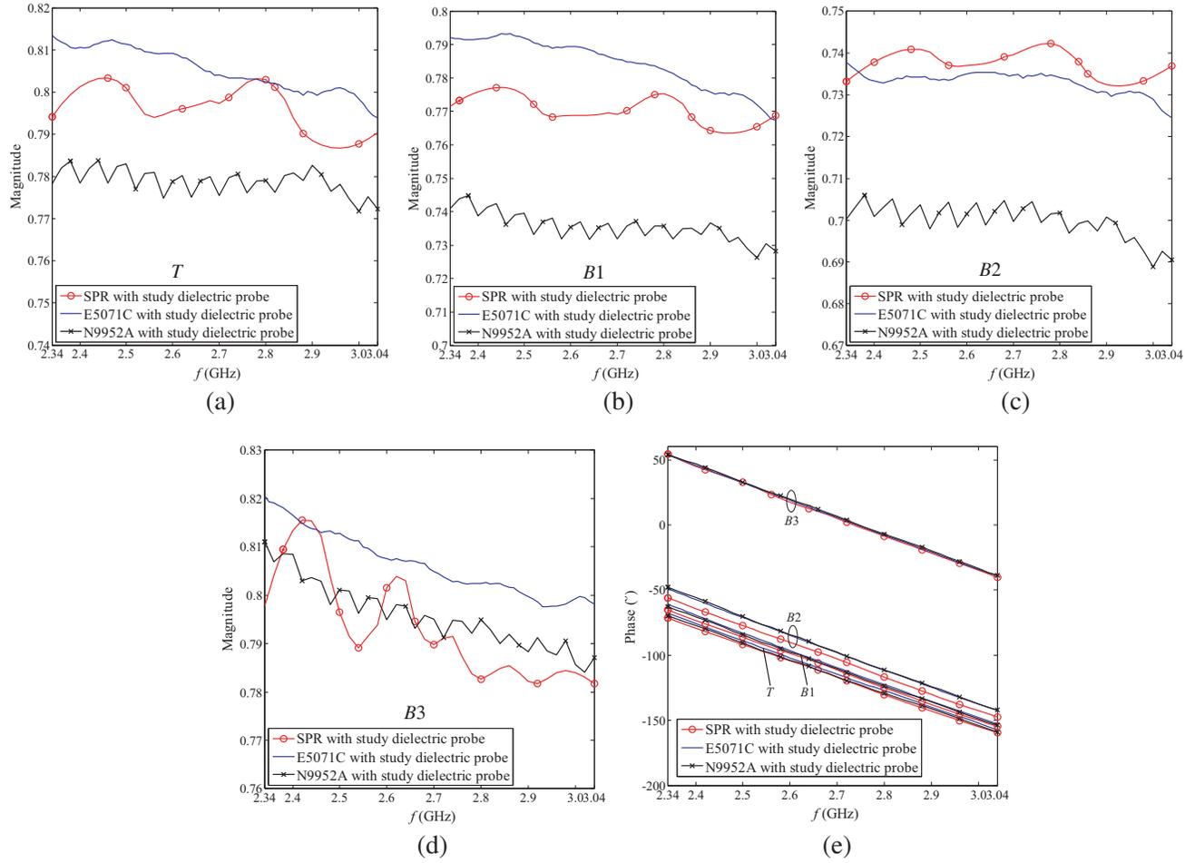
**Figure 11.** Measurement, (a)–(d) magnitude, (e) phase of SPR, E5071C VNA and N9952A VNA with three normal ( $B1$ ,  $B2$ , and  $B3$ ) and tumor breast tissues ( $T$ ).
