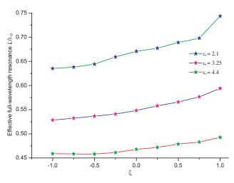
Figure 8. Effect of chirality on full-wavelength resonance for various dielectric constants  $\varepsilon_r$ .
