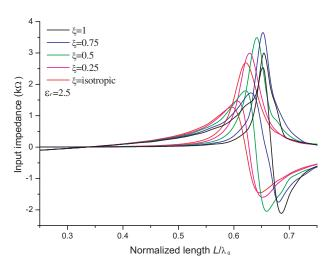
Figure 6. Positive-chirality effect on the input impedance of bi-isotropic chiral dipole antenna,  $W = 0.01\lambda_0$ ,  $d = 0.0796\lambda_0$  and  $\varepsilon_r = 2.5$ .
