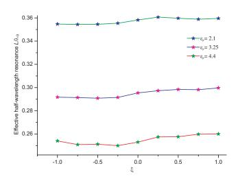
Figure 7. Effect of chirality on half-wavelength resonance for various dielectric constants  $\varepsilon_r$ .
