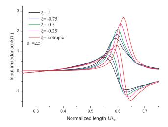
Figure 5. Negative-chirality effect on the input impedance of bi-isotropic chiral dipole antenna,  $W = 0.01\lambda_0$ ,  $d = 0.0796\lambda_0$  and  $\varepsilon_r = 2.5$ .
