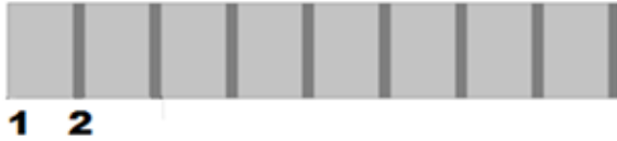
Figure 1. Dielectric photonic crystal: 1 — quartz layer with the thickness d_1 , 2 — silicon layer with the thickness d_2 .
