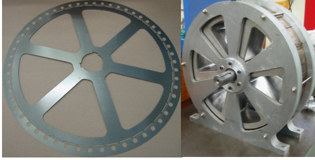
Figure 12. Lamination of rotor and stator prototype and the constructed prototype machine.
